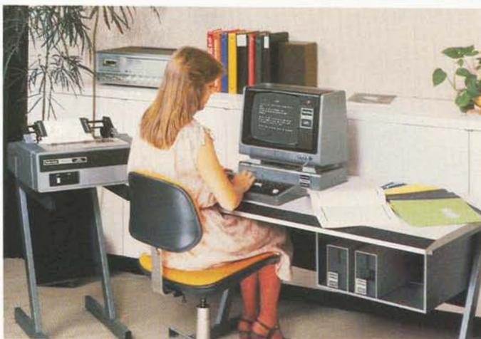
Approximately 135,600 bytes of disk storage space from the two mini-disk systems. Tractor feed line printer uses fanfold paper with feed holes in the margins and will produce up to 5 carbon copies. The System Desk has recessed spaces for the Expansion Interface and keyboard with interconnecting wiring concealed. Line printer stand leaves more desk space.
