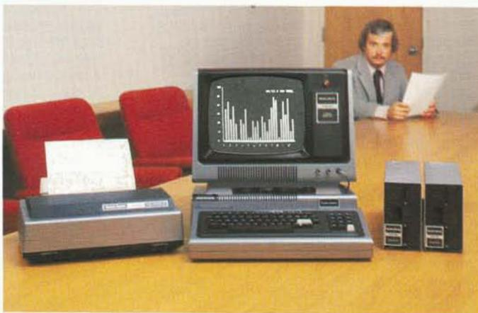
Two mini-disk units give user approximately 135,600 bytes of disk storage. Virtually all TRS-80 disk-based business software requires this as a minimum system. Applications include general ledger, payroll, disk mail list and more. Line Printer II adds real versatility and convenience to this system, without taking up a lot of work space.
