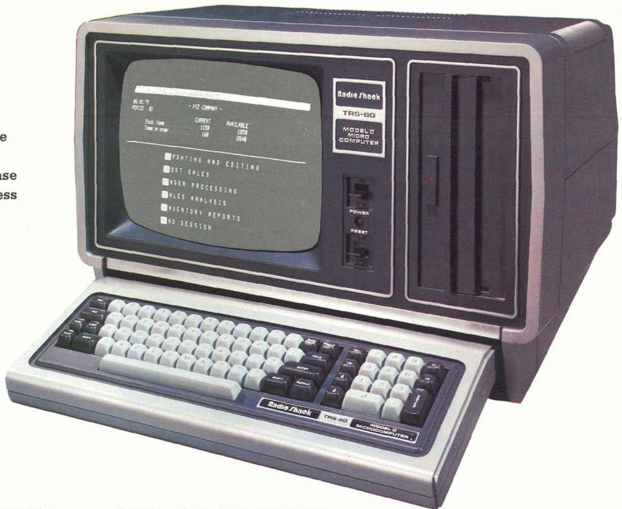
Anyone accustomed to a typewriter will feel right at home at the Model II keyboard. We kept it simple, with as few "special" keys as necessary to do the job. A calculator-style keypad is provided for faster, more accurate numeric entry. Model II's easy-to-read 12-inch, high-resolution video screen displays 24 lines of 80 upper and lower case characters per line. (Double-width characters—40 per line—can also be selected by your program).
