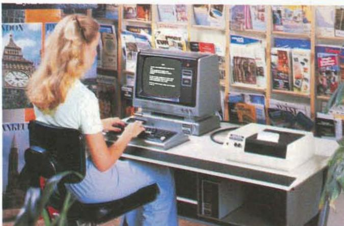
Mini-disk for expanded language, fast data handling and approximately 49,900 bytes of user disk storage space. Quick Printer provides 80-column hard copy and program listings. System Desk holds the entire system with plenty of work space left over.
