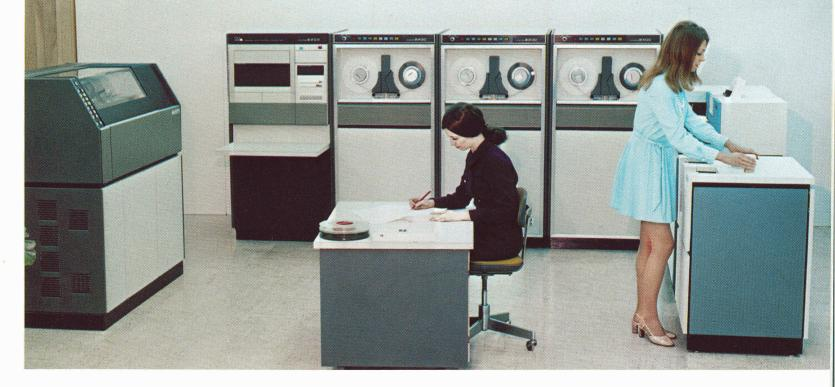
Blocked magnetic tape is the least expensive input medium. Converting from punched cards, punched paper tape, unblocked magnetic tape, and so forth to blocked computer tape on the main frame is costly.
