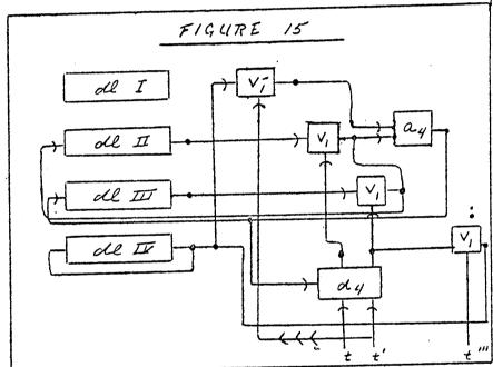
radicand is originally in dl III, but is replaced, as the square rooting progresses, by the successive partial remainders. The valve  $v_1$  routes the square root a (as formed up to that position) negatively into the adder—the timing must be such as to produce a shift left, thereby replacing a by 2a, and the absence of the extra correcting pulse for subtraction (t" in Figures 11 and 13, cf. the discussion above) replaces it by 2a+1. The two valves  $v_1$  immediately under it select the partial
