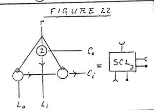
supposed to come from C, goes on to  $L_i$ , and  $L_o$  is isolated from all connections. Hence SCL produces the first state of 13.3 when r is not stimulated, and the second state when r is stimulated. We also note, that in the first case a stimulus passes from  $L_o$  to  $L_i$  with a delay 7 (cf. the timing question of  $SG^1$ , discussed above.)
