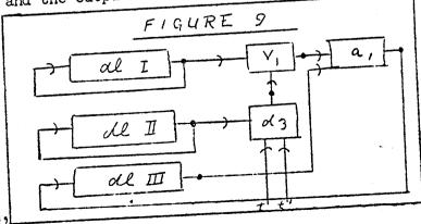
and the sum of partial products (which begins with the value 0 and is gradually built up to the complete product) through dl III. The two inputs t, t' receive the timing stimuli required by the discriminator (they correspond to t, is in Figure 8.).
