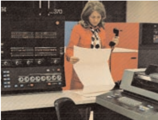
System/370, announced in June of 1970, introduced fully integrated monolithic memory.
