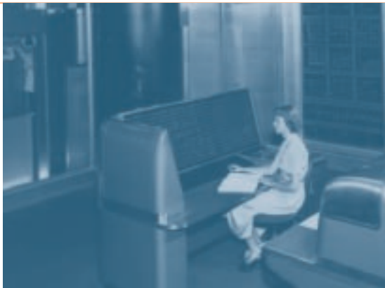
IBM's SSEC super calculator pointed up a critical problem: electro-mechanical input, output, and memory sources could not keep up with the new computing speeds.
