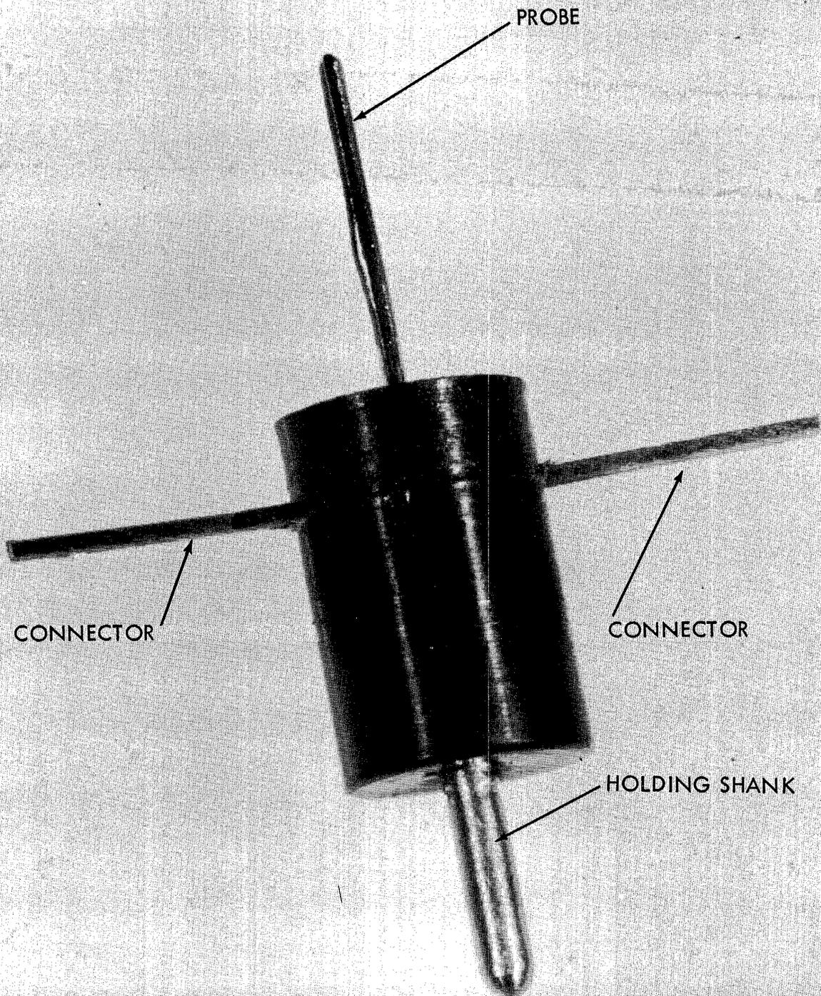
FIGURE 1 TWO CONDUCTOR PROBE FOR 30-50-12 TOROIDS
