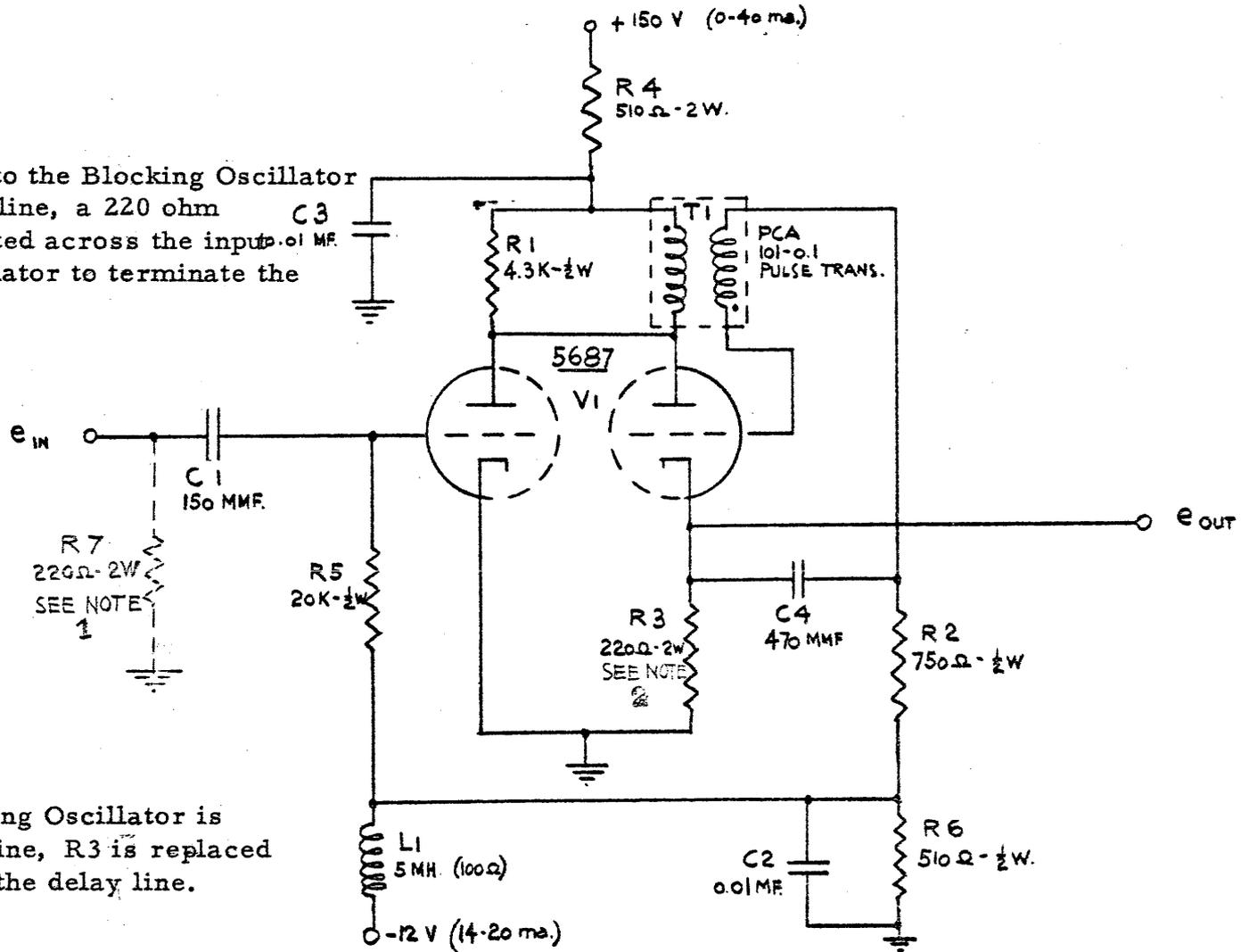
Note 2: When Blocking Oscillator is followed by a delay line, R3 is replaced by  $Z_0$  (220 ohms) of the delay line.
