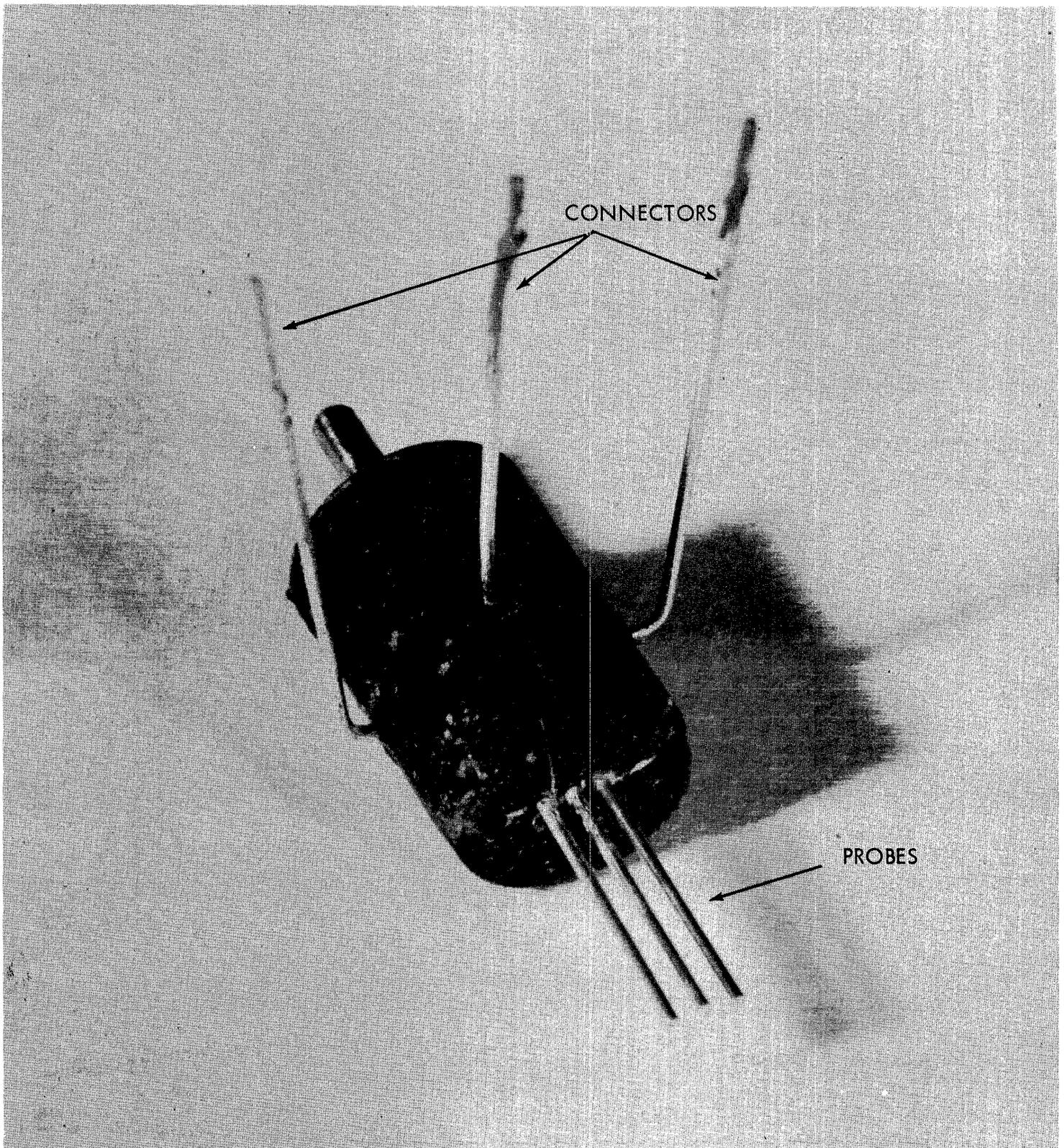
FIGURE 3 - 3-HOLE PROBE
