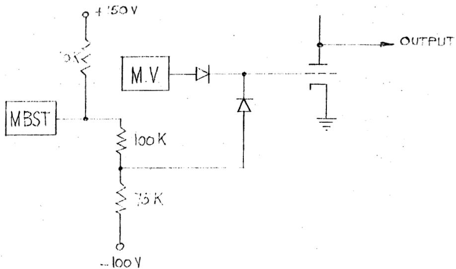
Consider the operation of the logic circuits as a whole. Multivibrator pulses are waiting to get through the 5 "and" gates. An output of the MBST is fed to an "and" gate. The gate is opened. The multivibrator pulses are fed to the grid of its respective amplifier. The signal
