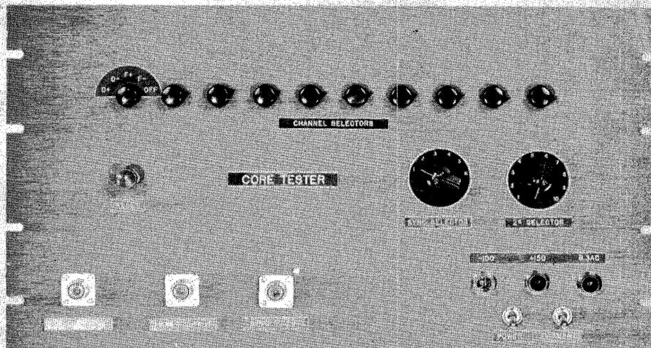
FIGURE 1 E - LOGIC PROGRAMMER FOR MODIFIED SKL #503 PULSE GENERATOR
