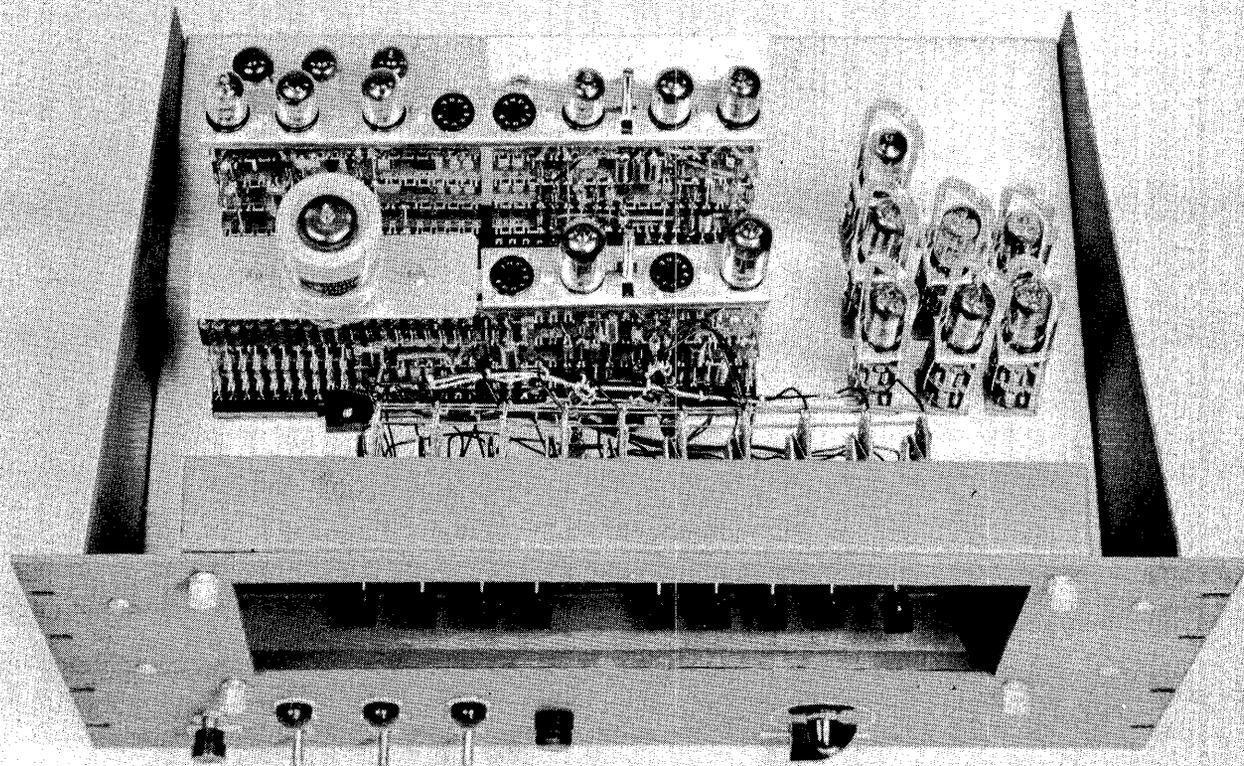
FIGURE 1 D - DRIVER LOGIC UNIT
