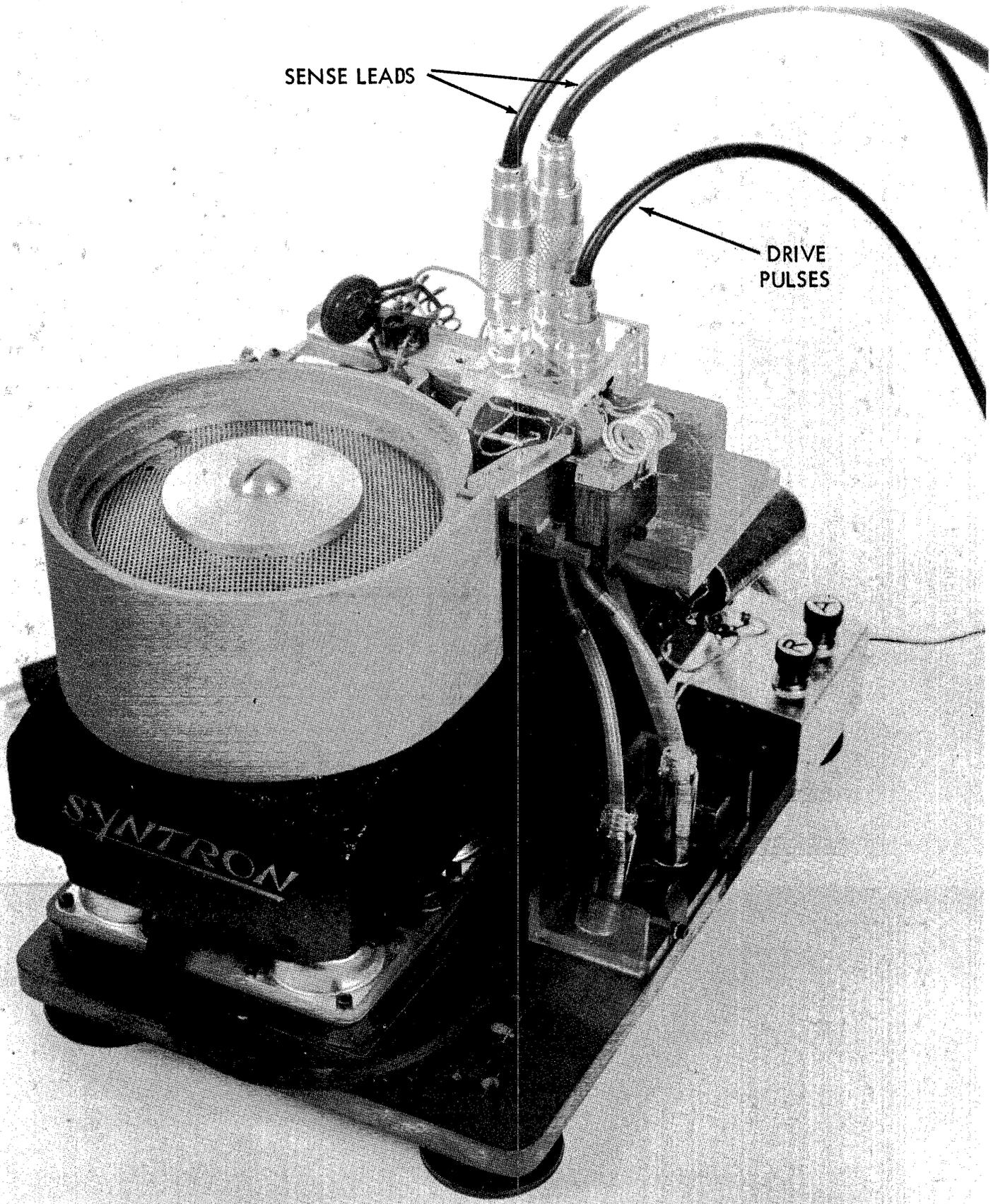
FIGURE 2 - AUTOMATIC 3-HOLE CORE HANDLER
