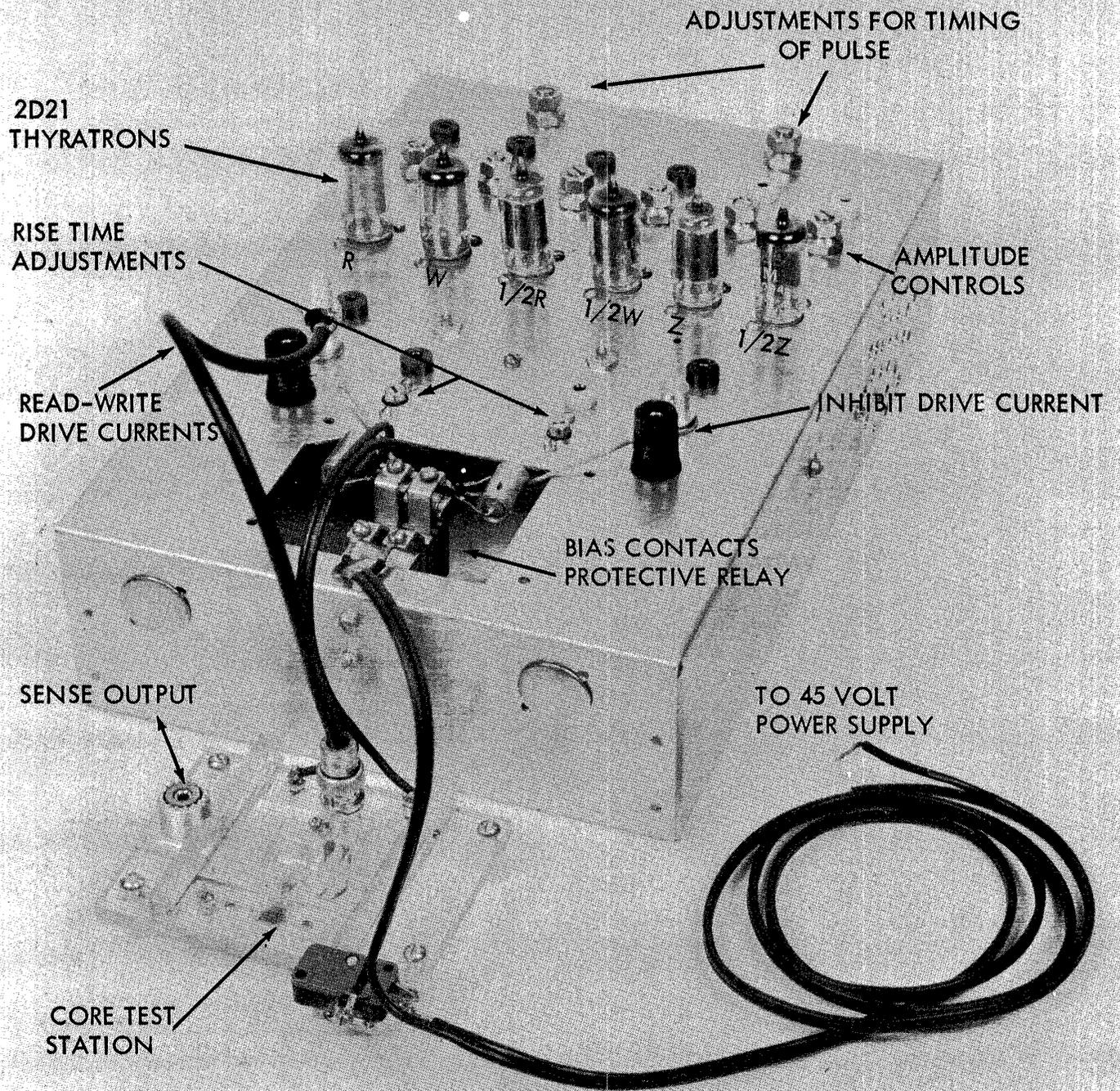
FIGURE 1 F - FAST RISE TIME DRIVERS WITH MANUAL 3-HOLE CORE TEST JIG
