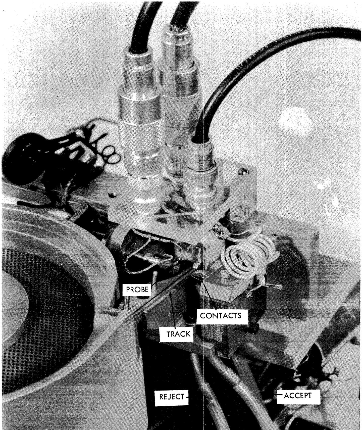
FIGURE 4 - 3-HOLE PROBE AND CONTACT ASSEMBLY
