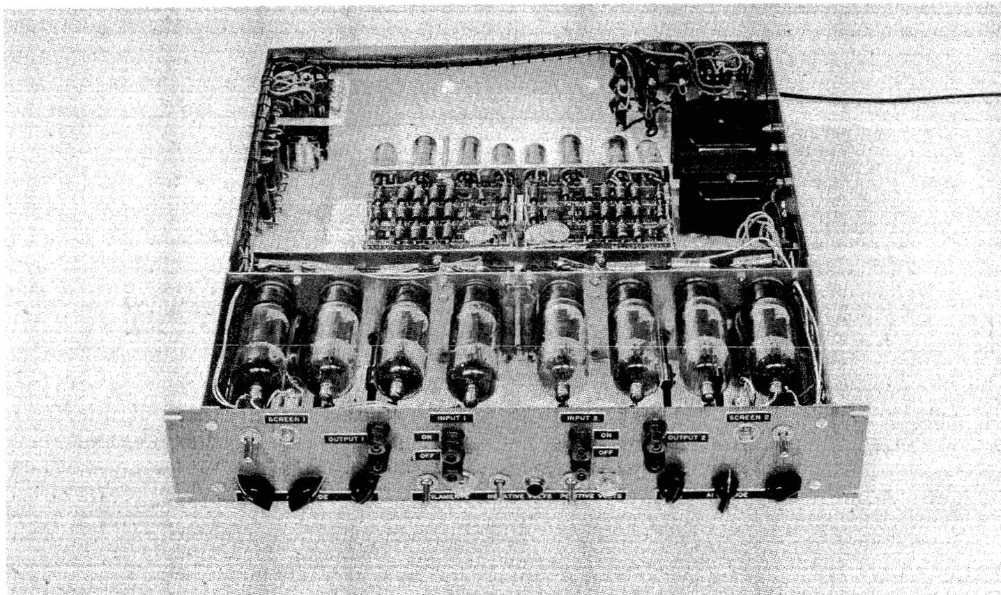
FIGURE 1 G - TWO CHANNEL CURRENT DRIVERS
