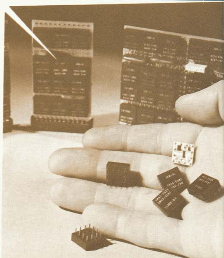
leave a logic card via contacts that connect to pins on a circuit board. Each logic card provides printed conductors for distributing voltages and signals between module circuit points and card pins.
