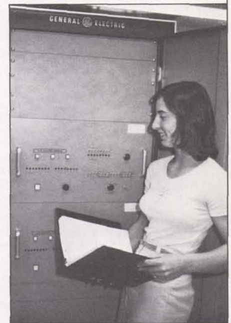
Christine Intihar, Background Computer Operator, Brook Park, examines a new ISBD bus adapter. Although only about a third the physical size of the bridge it replaces, its capabilities are far greater.
