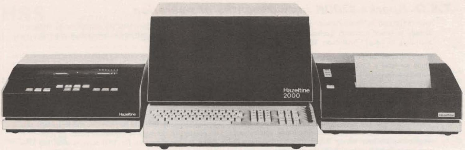
*Hazeltine 2000 with Dual Magnetic Tape Cassette and Thermal Printer.*
