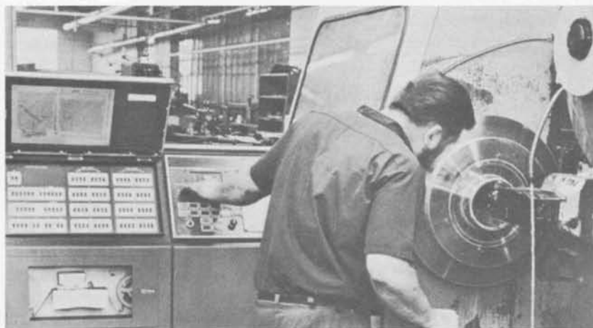
NC program, prepared on remote computer through time-sharing terminal, operates numerically-controlled lathe and gives small shop, big-shop capability.
