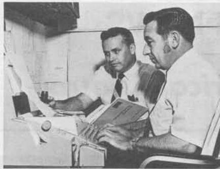
**2.** Time-sharing service with a library of over 500 programs related to all phases of business and industry aids an Armco Steel N/C programmer in producing a machine tool tape.
