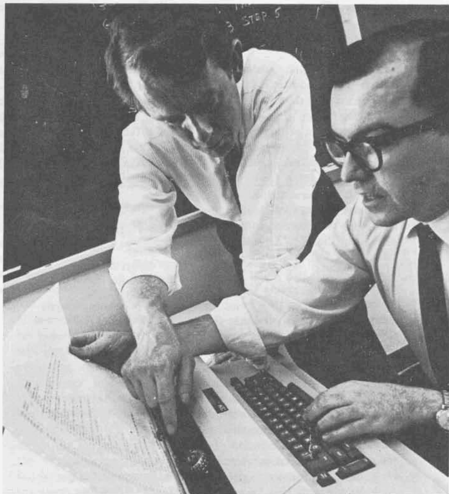
IBM's latest entry in the time-sharing picture, CALL/360:BASIC, combines the BASIC language with telephone access to a System 360 Model 50.
