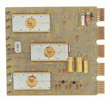
Large-Scale integrated circuit boards are the brains of the TermiNet 300 printer. These plug-in modules, the latest in electronic circuitry, make the printer more compact, easier to maintain.
