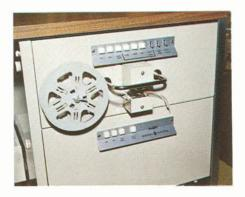
The tape reader is versatile in a number of other ways. It can read or omit the next character, word, or line by simply pushing the appropriate buttons. The reader can be backspaced and the tape can be rewound from either a remote or local location.
