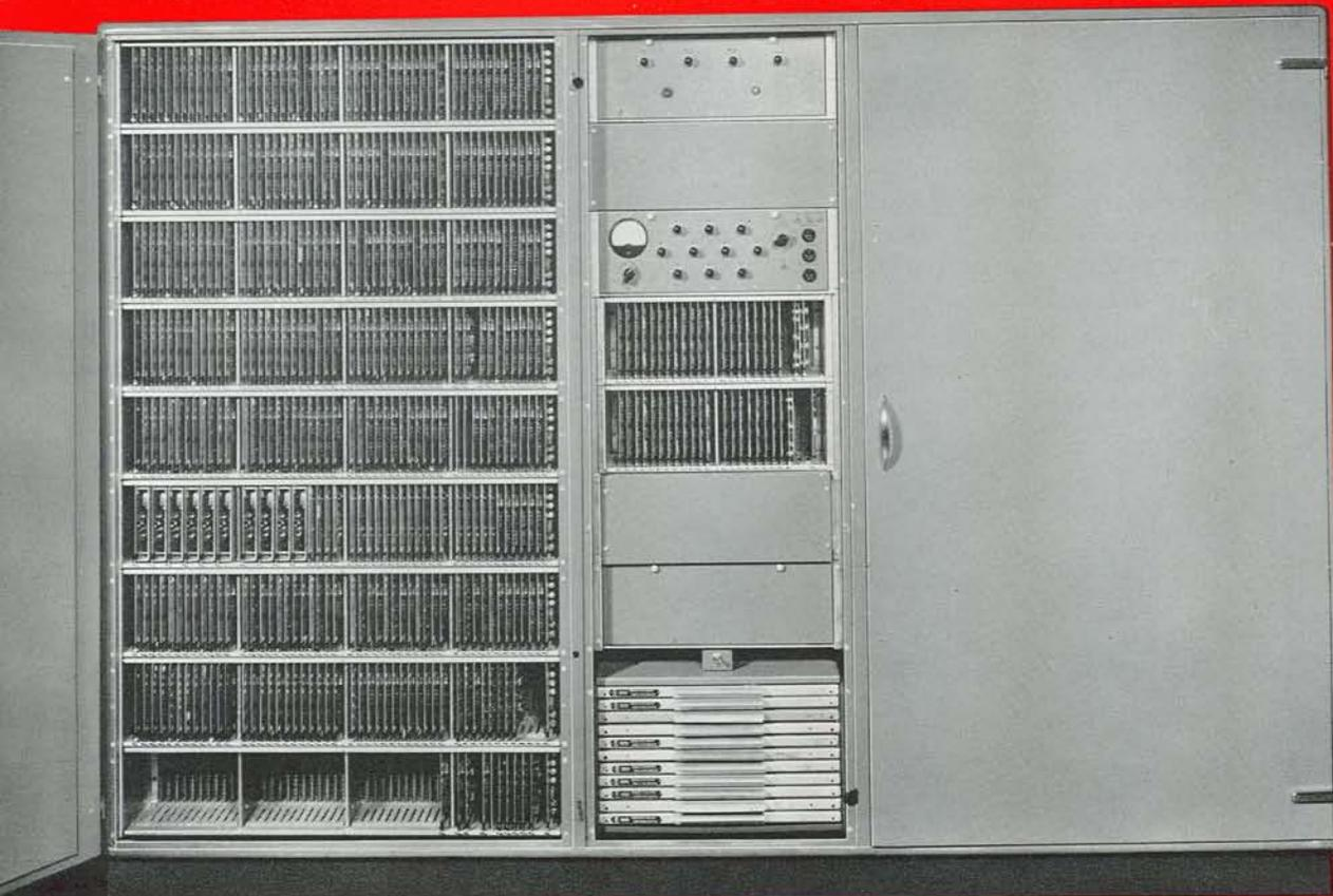
REAR VIEW OF SIRIUS. The delay line trays are at the bottom of the centre compartment and the accumulator packages are on the fourth shelf up at the extreme left.
