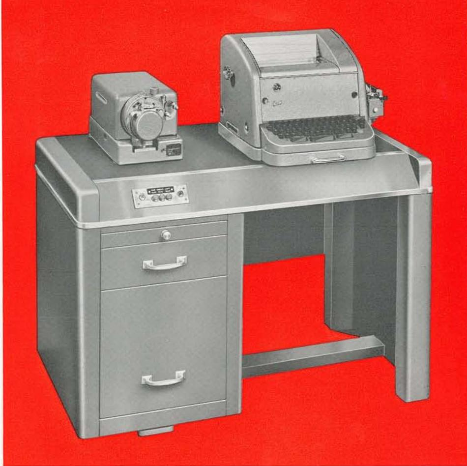
TAPE EDITING EQUIPMENT. The Creed 75 teleprinter shown may be used for tape preparation and for printing out results.
