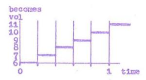
Accented notes may be coded by including the letter "v" anywhere in the note. This causes the volume of the note to be raised two volume levels for a duration depending on the note duration as shown in the following tables
