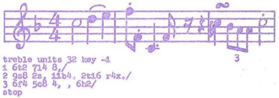
To run the compiler, load a copy of "mcomp" from Dectape O and start it at O or 102. The compiler expects the input text in Expensive Typewriter's text buffer. It places the output on the drum, where it should be saved on a Dectape using a standard file system.
