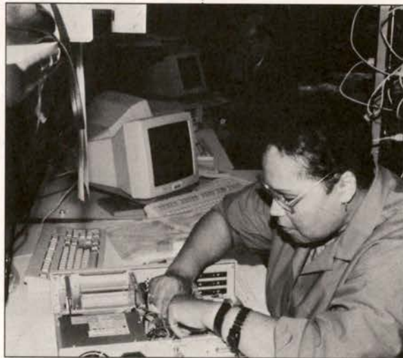
A SPRINGFIELD EMPLOYEE ASSEMBLES THE NEW DECPC LOW PROFILE PERSONAL COMPUTER. SPO IS THE ONLY REGIONAL ASSEMBLY SITE IN THE U.S. FOR THIS COMPUTER FAMILY.
