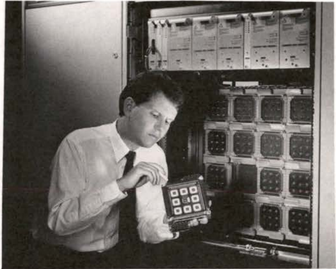
Tom Daley, a senior Customer Service support engineer, examines the Multi-Chip Unit (MCU) taken from the planar module of Digital's new VAX 9000 mainframe computer system. The MCU and the planar module represent breakthroughs in semiconductor packaging technology incorporated in the new computer.
