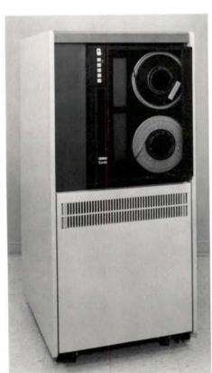
data checking on a single pass. An automatically activated erase head operates on writing.
