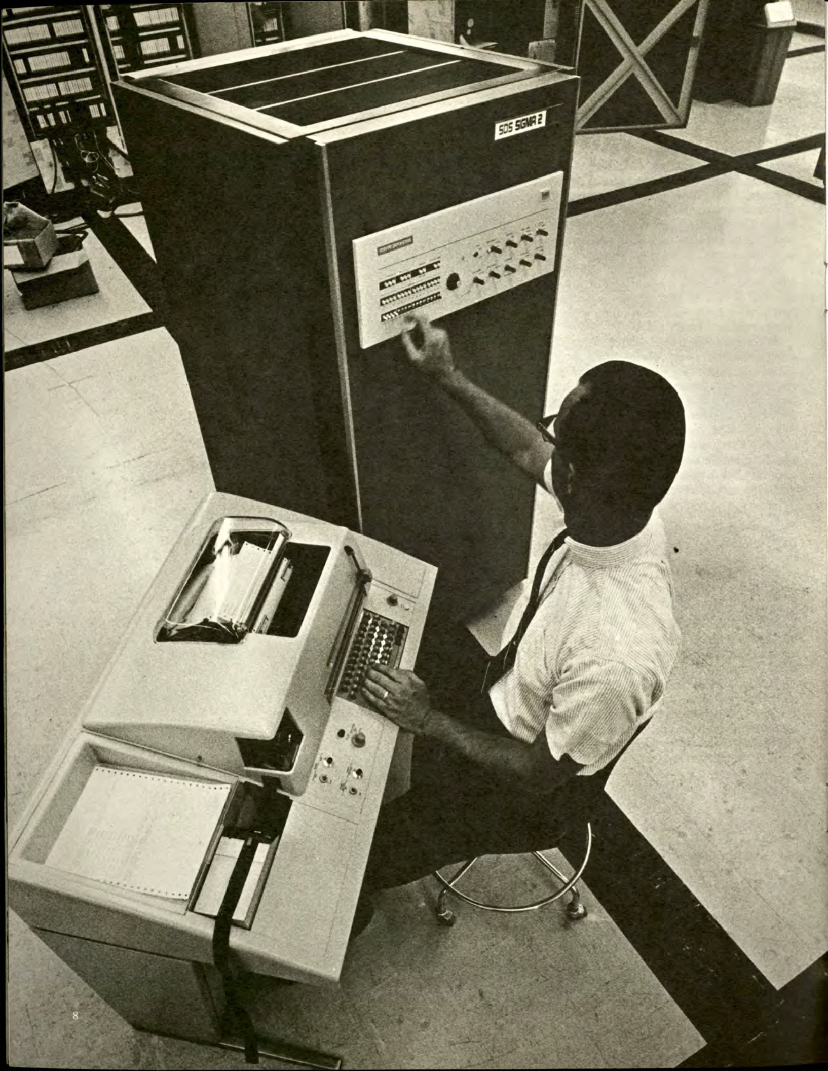
SDS engineer checks out low-cost Sigma 2 computer, which performs concurrent foreground/background processing.
