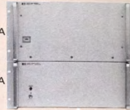
DISC MEMORY (2116B, 2115A only) 32 tracks, head-per-track 2720 addressable sectors 64 words/sector 174,080 16-bit words (64-track disc also available)
