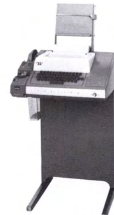
TELEPRINTER Keyboard, punch, read, print 10 char/sec ASCII character set
