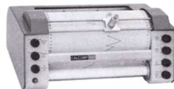
PLOTTER 300 steps/sec Resolution .01 inch Plotting width 11 inches
