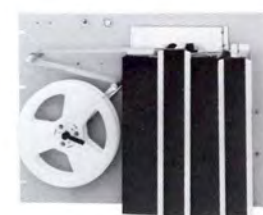
TAPE PUNCH Punches 8-level code 120 char/sec
