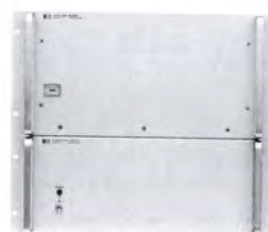
DISC MEMORY (and power supply) 32 tracks, head-per-track 174,080 16-bit words
