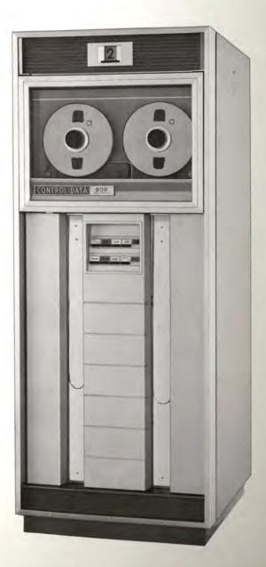
tape load and unload procedures is provided by a bank of operator keys and status indicators. Tape changing is simplified by straight line threading and the use of leaderless tape which requires but a single wrap on the take-up reel. Industry and system compatibility is maintained by use of 101/2 inch reels and IBM standard EOT and BOT-load point reflective spot sensing.
