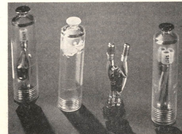
Fig. 21 (right). TX-0 logic units
