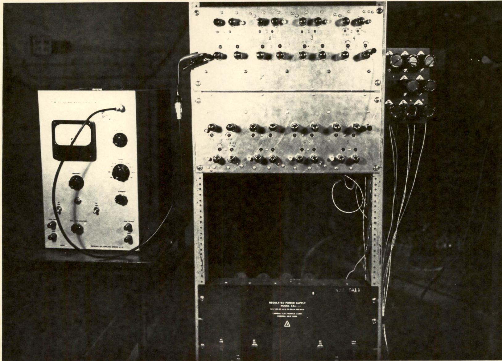
FIG.14 FRONT VIEW OF ENCODER AND SQUARE WAVE GENERATOR
