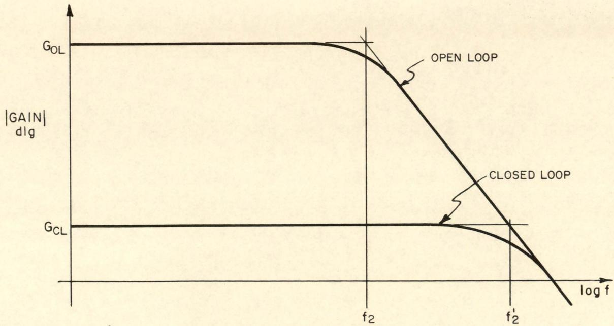
Fig. 8 Open and Closed Loop
