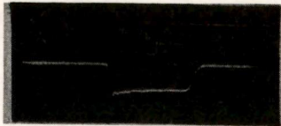
FIG. B9 CORE DRIVER OUTPUT CURRENT (THROUGH 10Ω LOAD) WHEN INPUT PULSE AT 1 IS TOO LARGE
