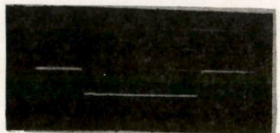
FIG. B12 1.8μ SEC CORE DRIVER OUTPUT PULSE
