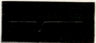
FIG. B11 0.1μ SEC CORE DRIVER OUTPUT CURRENT PULSE
