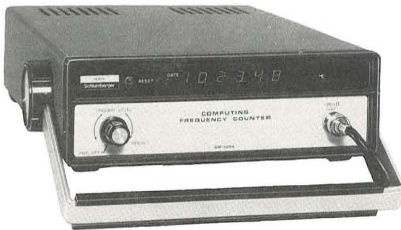
Figure 10-7 A computer frequency counter measures period then computes frequency to provide high measurement resolution at low frequencies.
