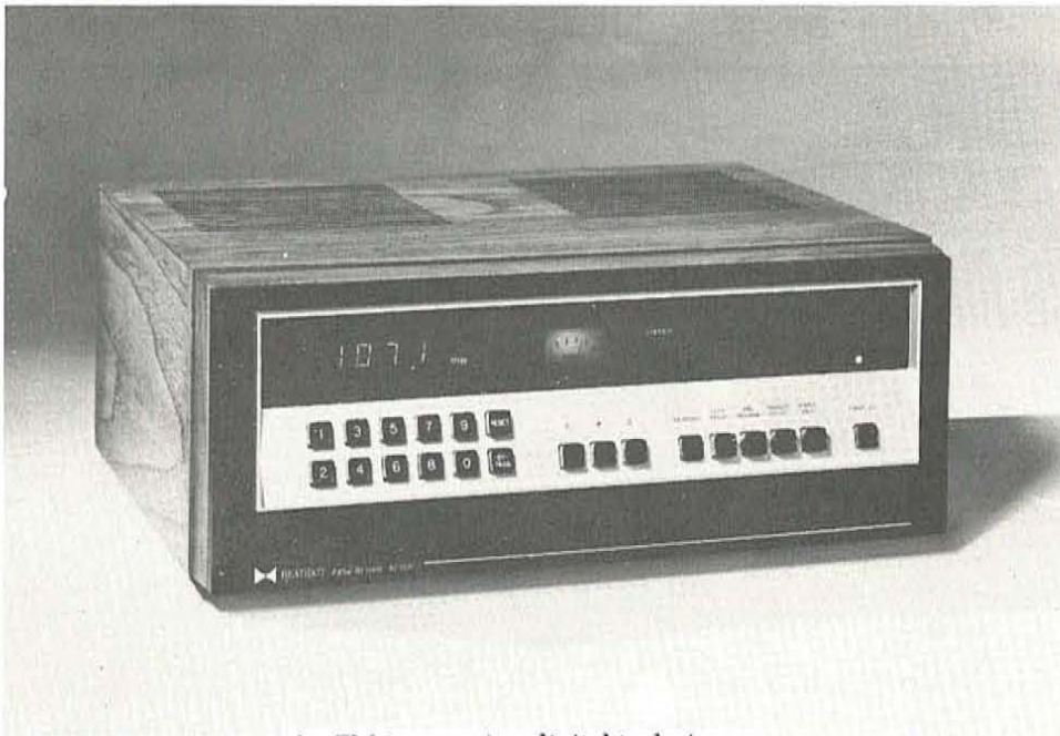
An FM tuner using digital techniques for frequency selection and display (Heath Co.)
