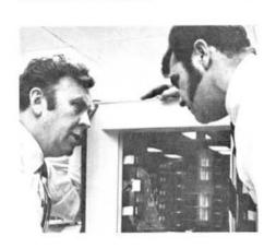
Developed by SDD San Jose, the fastest auxiliary storage unit in the company's product line -- the IBM 2305 Fixed-Head File -- is announced. The new file employs a total of 768 magnetic heads to achieve its high-speed average access time of 2.5 milliseconds. Discussing the development model are SDDers who worked on the 2305 project, Henry G. Hoehmann (left), mechanical design manager; and Mark M. Burd, technical associate, electrical development.
