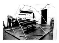
Design of a new building for Research begins. Research personnel constructed this "sun model" which could simulate the lighting effects of the position of the sun for any hour of any day of the year.
