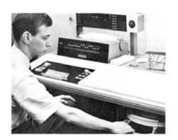
The first IBM 1130 computing system built in San Jose is installed at NASA's Huntsville, Ala. facility where engineers and researchers will use it in support of NASA's Saturn launch vehicle lunar program. Joseph W. Parks, assigned to the Marshall Space Flight Center, installs a removable disk cartridge in the new computer.
