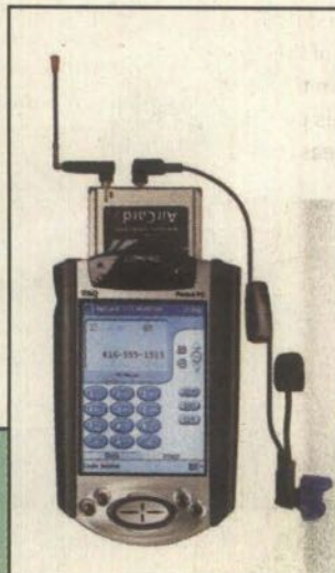
A PC Card-equipped handheld allows users to make voice calls and send and receive email wirelessly using CDMA (like this Telus combination) or GPRS networks.
