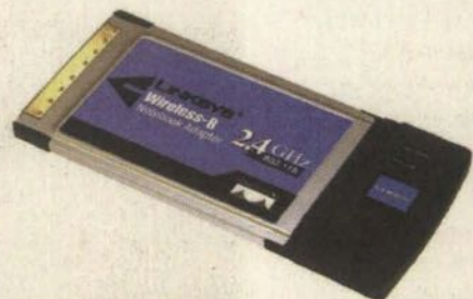
A PC equipped with a wireless card (like this one from Linksys) can connect to the Internet and network printers wirelessly within range of a wireless hub.
