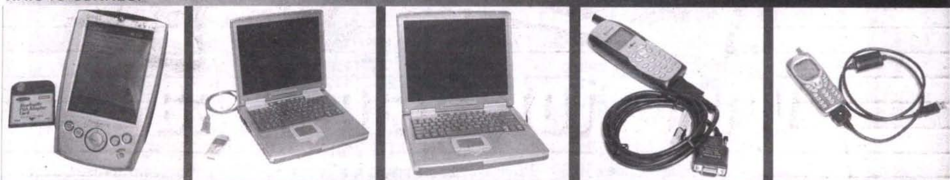
Bluetooth: A Pocket PC PDA with Bluetooth card (left) and laptop with Bluetooth dongle and Bluetooth phone (right).
