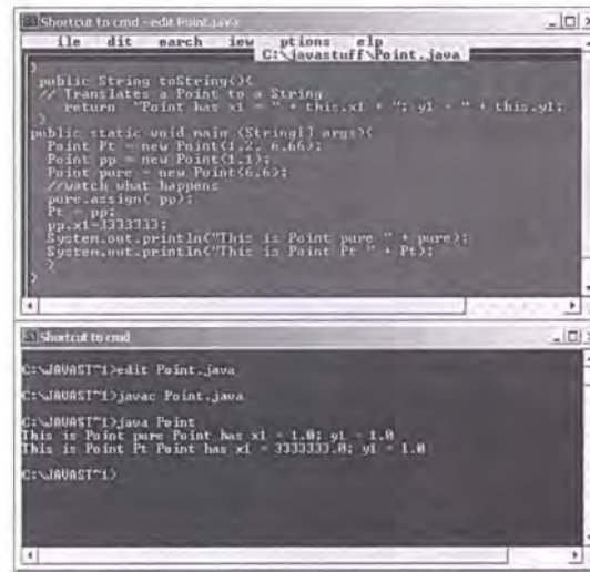
Fig. 2A (top) and Fig. 2B (bottom): Assignment statement gone awry in Java.
