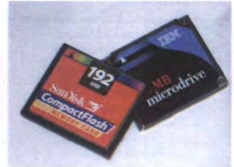
IBM's microdrive (left) is the size of a CompactFlash card and stores up to 1 GB of data.
