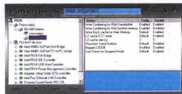
The PowerTweak control panel shows Celeron register settings and PCI/AGP devices registered with BIOS.
