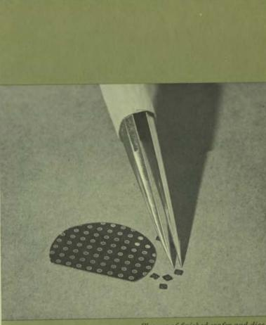
Closeup of finished wafer and dice
