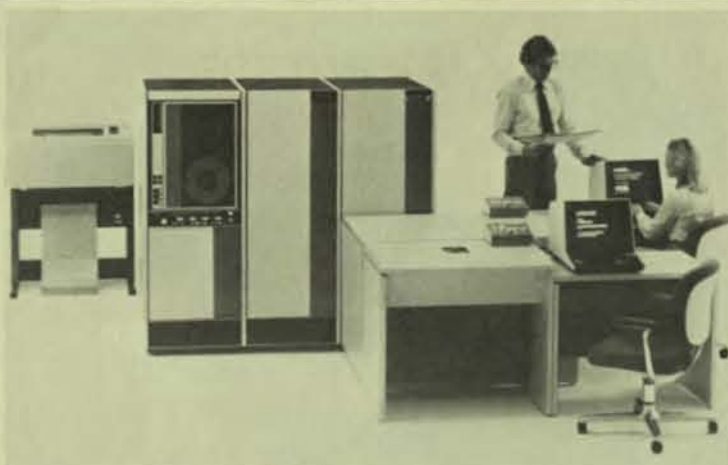
The new Sentry™ Series 20 was well-received by attendees and press at the Cherry Hill IEEE Test Conference in October. The fast, new LSI test system for microprocessors, memory chips and other high-speed devices, has been redesigned with more compact bays and smaller test heads for easy operator use.
