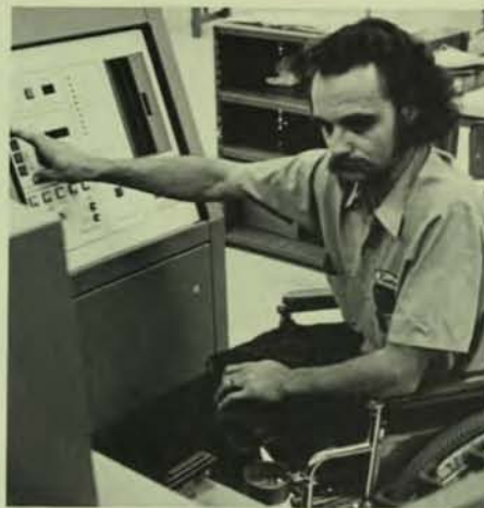
New electronic equipment, like this machine to automatically insert dozens of integrated circuits into printed circuit boards, gets a diagnostic run-through before being added to the production line at the San Jose Test Systems plant.
