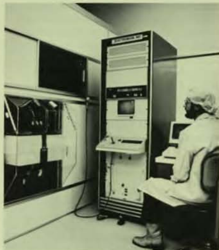
Dr. P. A. Crossley, a Senior Member of the Research Staff, works in the new VLSI laboratory in Palo Alto. He's operating a wafer stepper, which permits tighter tolerances and smaller geometries than any equipment used previously. It will be used to develop processes for the 256K RAM and other VLSI devices with feature sizes of less than two microns.
