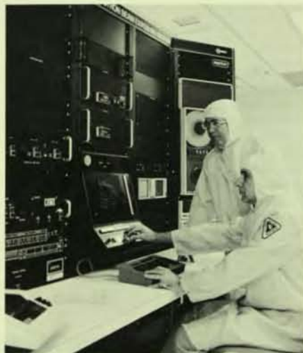
Vic Mitrising, Manager of Mask Making, demonstrates the new 40 megahertz electron beam mask maker, the only one of its kind in the world, for Jim Early, Manager of VLSI and Advanced Process Research.
