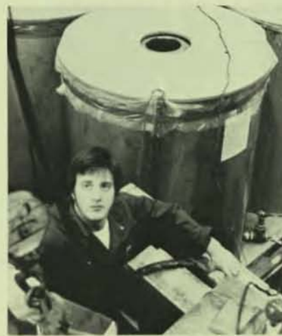
Cubes of rocks are packed into huge canisters to simulate an underground environment for testing new tools.
