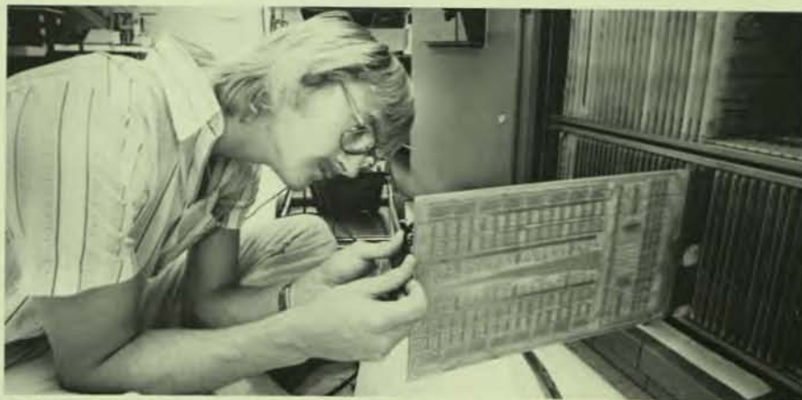
Problems in a tester can almost always be tracked down to a printed circuit board, says Field Support Specialist Jim Schraith.
