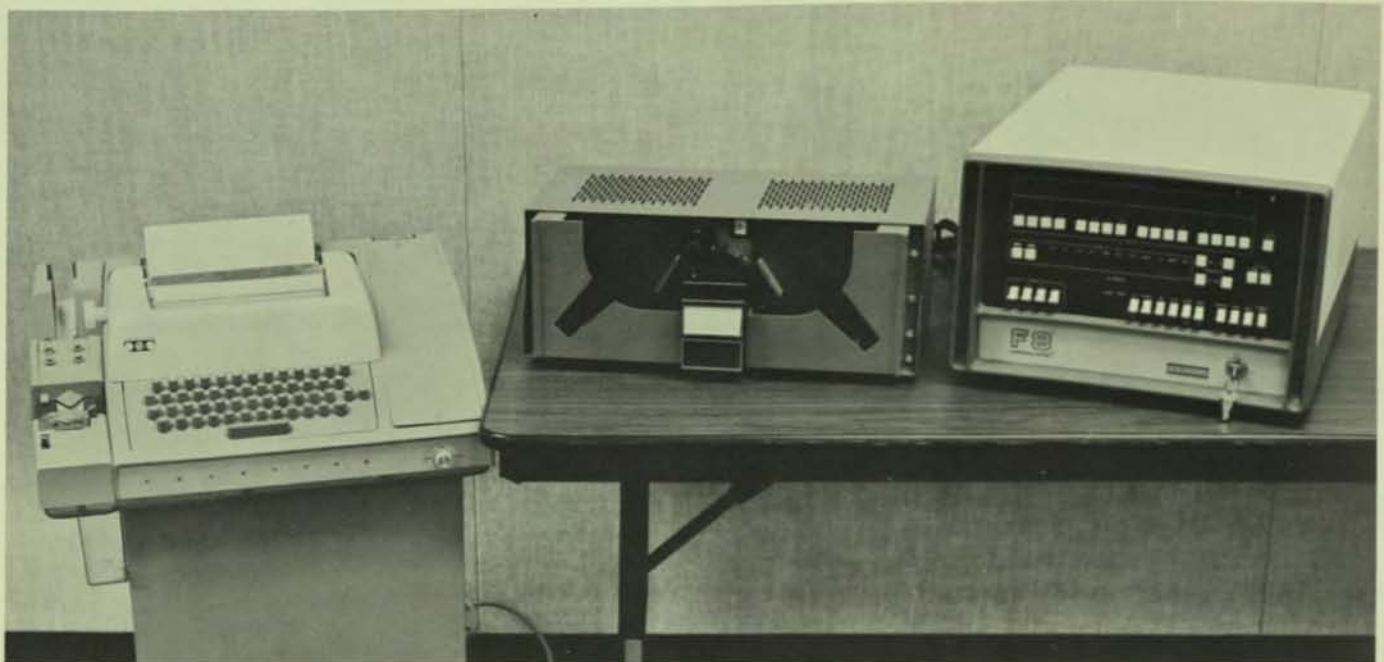
The F8™ FORMULATOR™ support system, shown above in a configuration including teletype equipment and a high-speed paper tape reader, is a design tool used in development of microcomputer-based systems from initial design through prototype development and testing. The FORMULATOR (inset below) is the system's central processing unit.
