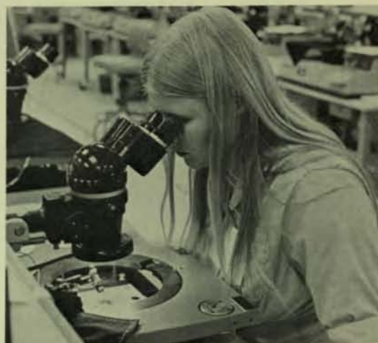
Kathy Bidner, wafer sorter in Analog Products Division, checks a wafer containing integrated circuit chips destined for Fairchild's voltage regulators.
