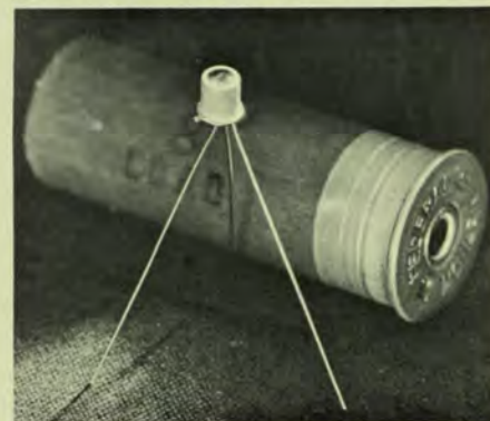
Pictured is a photo transistor in a TO-18 package. This unit consists of a standard 2N 699 transistor encapsulated in such a way as to allow light to strike the sensitive area.
