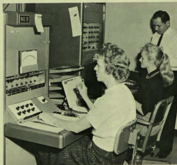
In the final testing area Mary Hendrix (left), and Beverly Tighe use a dc tester to check a sample of transistors from each outgoing shipment. Supervisor Ray Micotti is looking over final inspection results.
