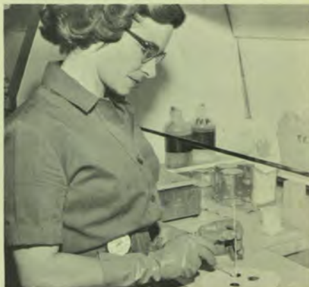
Pat Gavitt, metalizing, came up with an idea recently that is under consideration by the sustaining engineering group. Pat suggested that wafers be cleaned by pressing them on filter paper and then swabbing them with a cotton daub dipped in hydrofluoric acid, rather than waxing the wafers to glass slide in order to clean them. This saves the time and labor it takes for the waxing operation.
