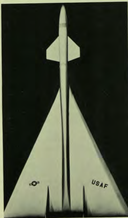
Special features of the Air Force B-70 Valkyrie, now under development, are shown in this view of a scale model. The aircraft, which will fly at three times the speed of sound, features small canard control surfaces near the crew compartment and large triangular wing surfaces.
