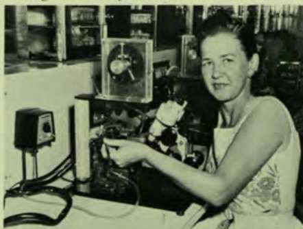
Lillian Mickey, assembler on the NPN line, demonstrates suggestion she made recently to improve the action on the lead bond machines. Lillian is pointing with pencil to the post where the adjustment was made. This has resulted in a saving of gold wire lead material and it also saves time and so increases the potential output of each lead bonder.
