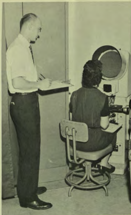
Marie Olsen operates an optical comparator, a device for precise measuring of dimensions, in the receiving inspection station where all material to be used in the fabrication of transistors is tested. Recording data is supervisor Ray Wollesen.
