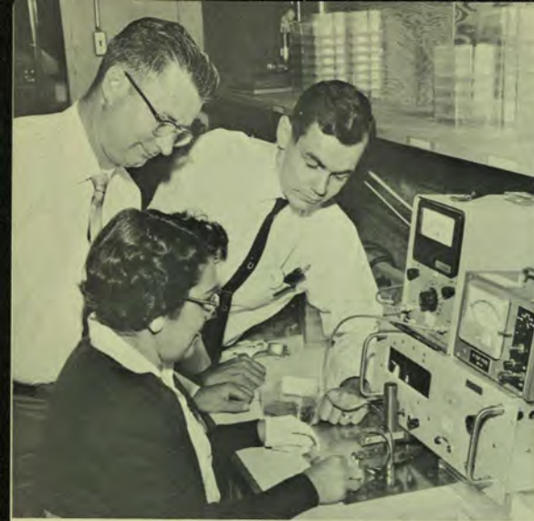
Ralph Ulrich (left) and Jay Cedarleaf survey their handiwork; Ralph adapted and assembled the digital resistivity tester shown and Jay developed the four-point probe with which operator Glee Klein is working.
