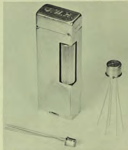
The chopper—a single package containing two transistors connected thermally with closely matched electrical characteristics.
