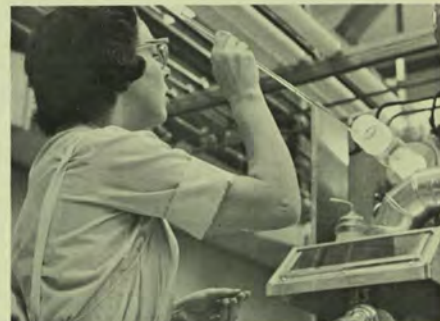
(B) Assembler Grace Gunter is putting a quartz "boat" of wafers into the diffusion furnace.
