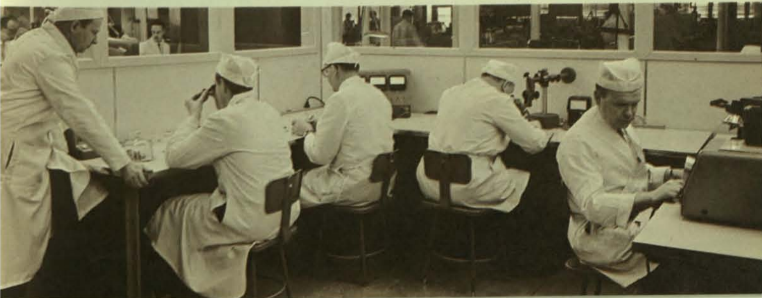
Fairchild Components are assembled under carefully controlled atmospheric conditions as in this gyro assembly "clean" room.
