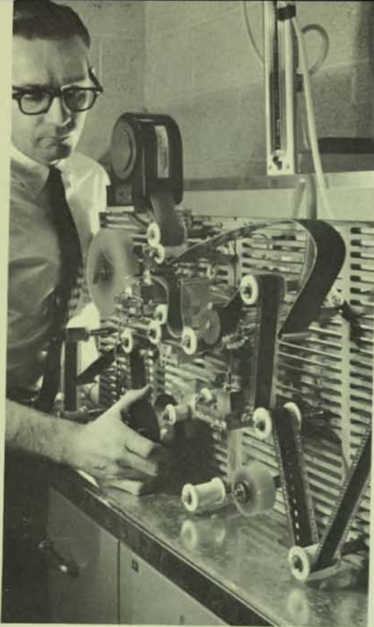
Fairchild is a pioneer in rapid film processing techniques. Model of rapid processing unit above is used for analyzing new approaches to viscous processing.
