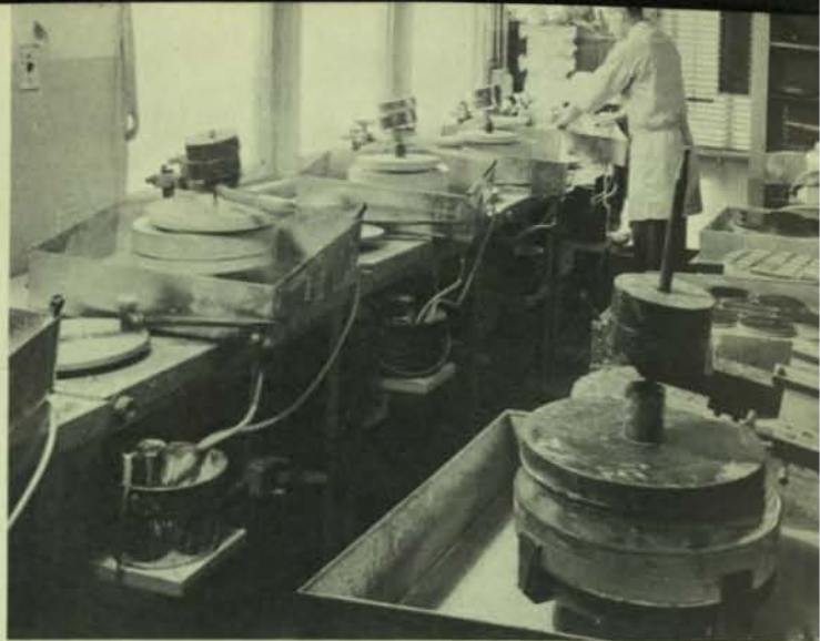
Grinding and polishing operations produce optics to the most exacting requirements at the Curtis Optical Department.
