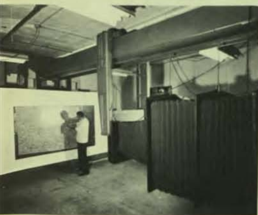
Aerial mapping and exploration call for many skills and varied complex equipment. From top to bottom are: Kelsh Plotter with Benson Lehner automatic cross section equipment installed; the drawing table of the C-8 Stereoplanigraph with cross section equipment in operation; and the giant copying camera used to photograph large mosaics and maps.
