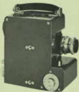
The Fairchild System Siemens (top) is a versatile 16mm recording camera designed for a wide range of laboratory and scientific photo applications.
