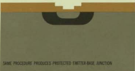
DIFFUSION SPREADS LATERALLY EQUAL TO DEPTH. OXIDE REGROWS DURING DIFFUSION
