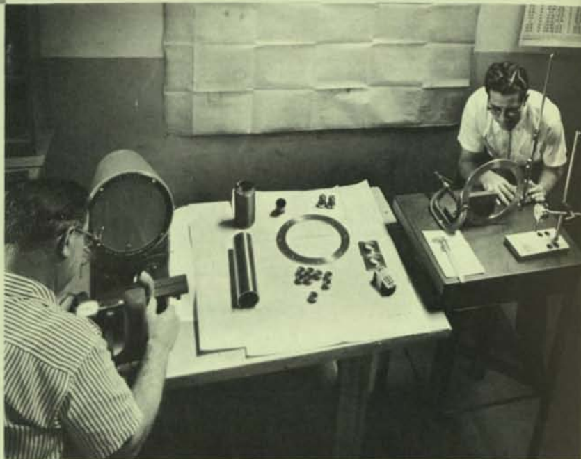
Quality Control at Special Products Division is maintained at a very high level. All critical parts, tube configurations, irregular profiles, etc. are constantly checked on a statistical quality control sampling basis.
