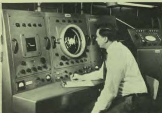
Du Mont Cathode-Ray Tubes are used in display indicators of new meteorological radar sets now in use by the United States Weather Bureau for more accurate and immediate weather forecasting.
