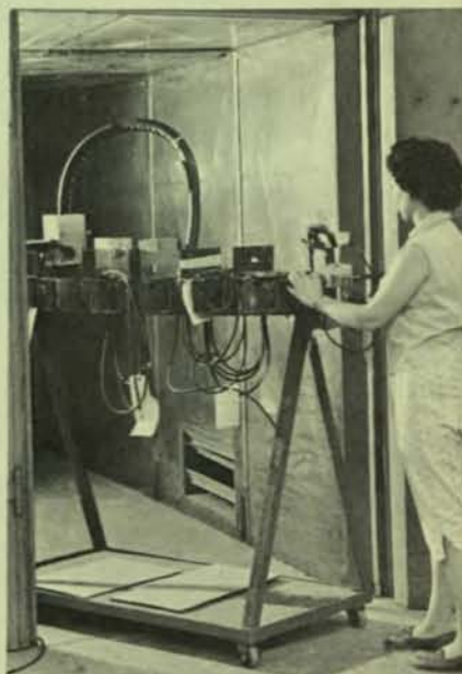
Molded cable terminations and connectors are cured in the plant's specially built ovens. Curing requirements vary with each type of assembly.
