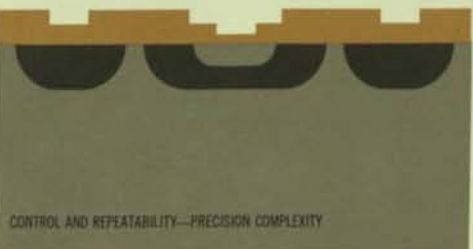
SAME PROCEDURE PRODUCES PROTECTED EMITTER-BASE JUNCTION
