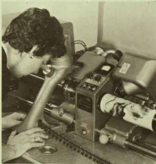
Teletypesetter equipment, which automates Linotype and Intertype linecasting machines has enjoyed world-wide acceptance. The Perforator Unit shown above uses a typewriter-like keyboard to punch tape from which the linecasting machine is operated automatically.
