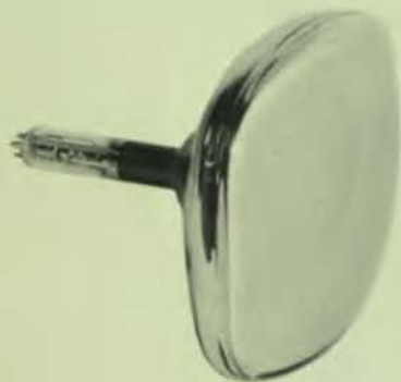
Top to bottom, the new Du Mont double-ended scan converter storage tube; an advanced design of an oscilloscope tube for modern instruments; and a new, lightweight, compact radar tube particularly suited for use in aircraft where weight and size are vital factors.
