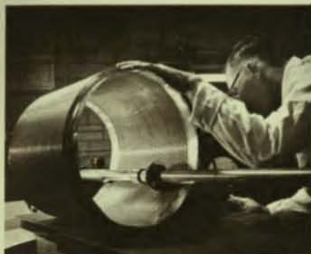
Fabrication of precision-formed lightweight metal products requires a high degree of manual skill. Mechanic is shown here performing extra stage spinning operation to deepen corrugations in a flexible member.
