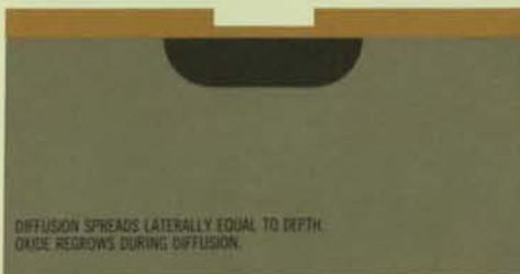
ETCHED OXIDE ALLOWS PRECISE LOCALIZED DIFFUSION OF IMPURITY
