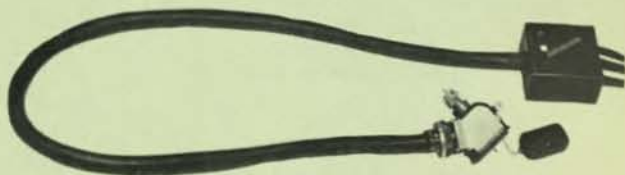
Another one of the TITAN umbilical cables. This assembly has 107 conductors and the molded junction alone weighs about 60 pounds.
