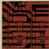
OPERATORS 9304 - Dual Full Adder/Parity Generator
