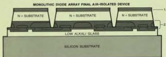
1. BONDING AREA 2. ACTIVE AREA WITH METALIZATION
