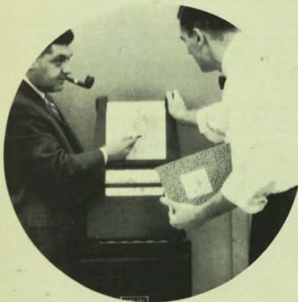
Facsimile receiver is shown here. With this equipment, drawings, printed data of all kinds, time sheets, inventory records, etc. can be transmitted and received over long distances in minutes.
