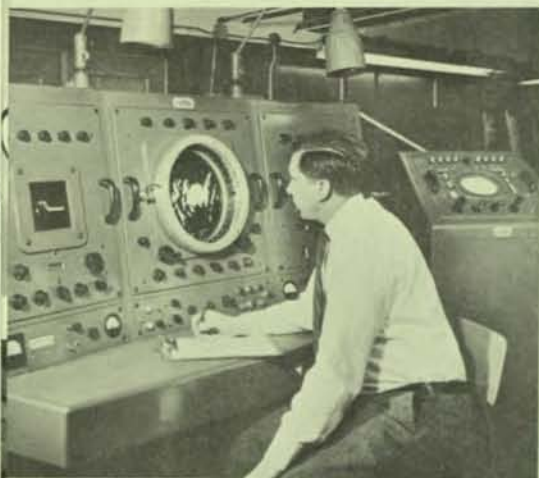
DuMont Enginoscopes (top) are standard at Ford Motor Company assembly plants. These versatile instruments provide an almost instant quality control check of engine performance.
