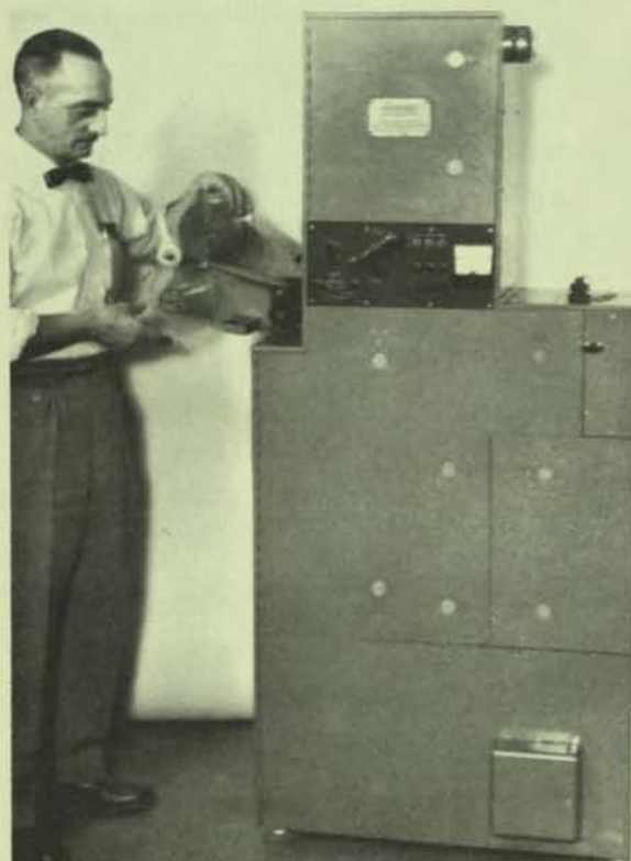
70mm Recorder-Processor—Utilizes new "Thixotrol" processing technique which permits continuous rapid processing of film as it is exposed. Designed to meet a Signal Corps requirement for rapid recording and viewing of cathode ray tube traces, film is developed within 10 seconds of exposure at speeds up to 90 feet per minute.
