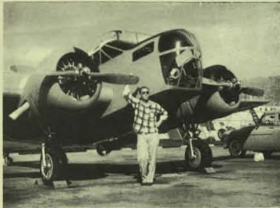
One of Fairchild Surveys' fleet of special photographic aircraft. Note the magnetometer which is attached directly beneath the airplane behind the man.
