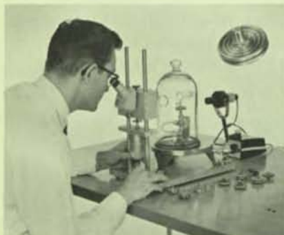
Above—Checking precision-formed aneroid capsule diaphragms for hysteresis, linearity and motion under vacuum bell jar. At right—Precision welding of wafer-thin materials is a specialty of this Division. Welder is shown here butt-welding thin wall stainless steel tube.
