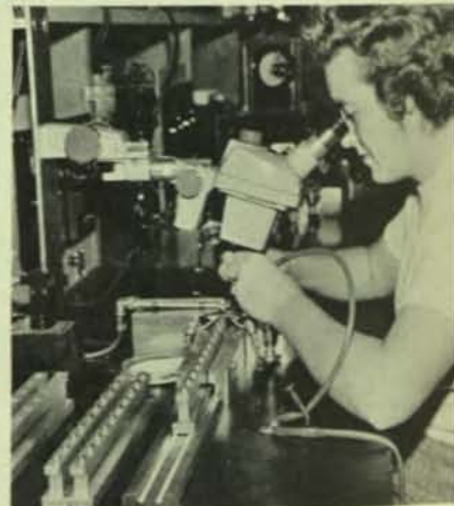
Transistor production has been expedited through elimination of much manual handling of tiny parts. This is a die attach station in which parts move on metal track past the operator.
