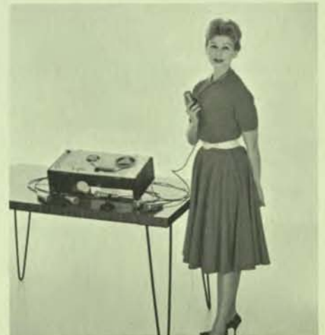
Below—Prototype model of new multi-channel voice recorder/reproducer. It is actually 6 recorders on one chassis.
