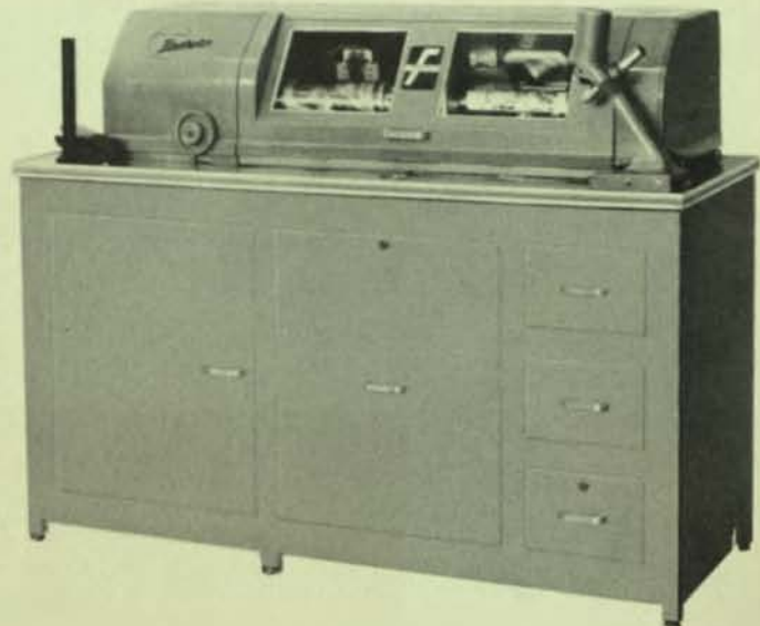
Continuing to offer the most advanced electronic halftone engraving equipment, the Graphic Equipment Division, in 1959, introduced the new Scan-A-Graver "Illustrator" shown here. Among its many new features, this machine provides the means for enlarging engravings directly from original photographs in two ratios as well as the usual 1 to 1 reproduction ratio.
