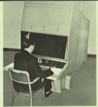
New Screening Viewer (above), developed and produced for U.S. Air Force, incorporates folded optical path rear-projection system for unimpeded viewing of photographic data on a 19 x 36 inch screen.
