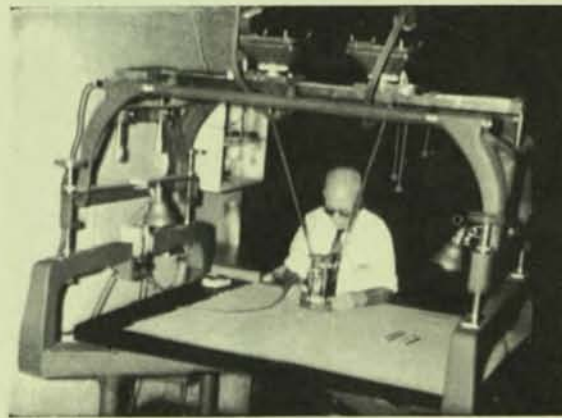
Another precision device for drawing contours is the Kelsh Plotter shown above. Like the Stereoplanigraph this is a stereoscopic plotting instrument.
