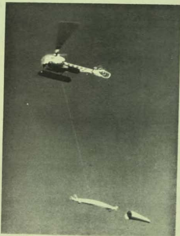
Another new tool employed by the Surveys Division is the Helicopter-borne magnetometer for use in making magnetic surveys for ore detection.
