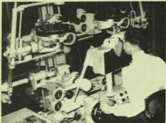
The Stereoplanigraph is a very complex and highly accurate stereoscopic plotting instrument used for producing contour or topographic maps from aerial photos.
