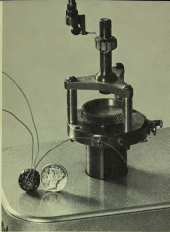
This tiny motor stator being wound on a special winding jig will eventually contain 10,800 turns of wire one-tenth the diameter of a human hair. The finished stator, when equipped with its rotor, will be capable of reaching speeds of 24,000 revolutions per minute in only ten seconds.
