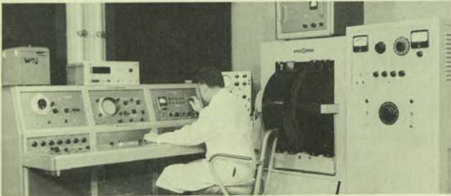
New Basic Research Laboratory of Defense Products Division is furnished with latest and most advanced test equipment. Shown here is a Magnetic Nuclear Resonance Spectrometer.
