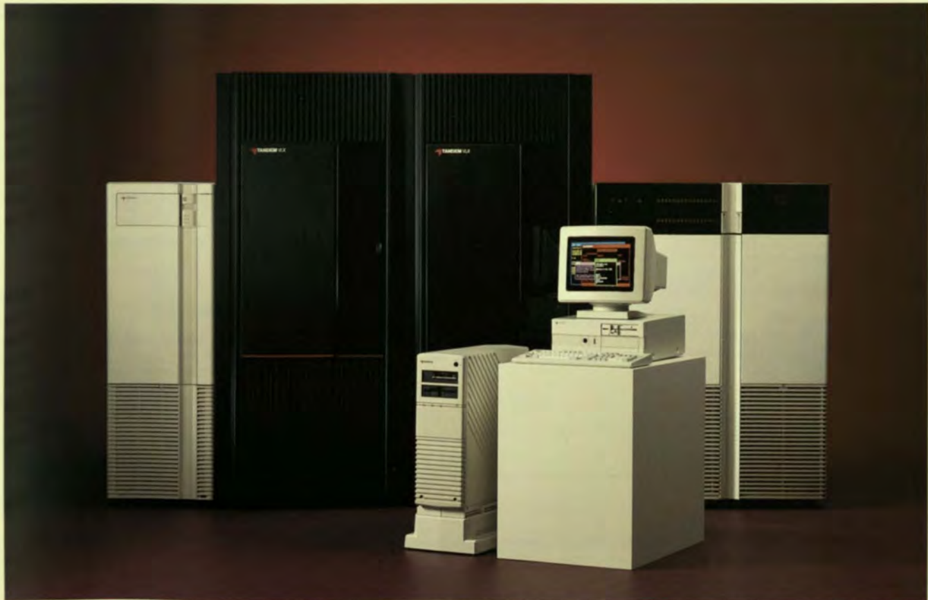
Shown above are some of the newer members of the Tandem product line. Clockwise, from left, are the NonStop CLX, NonStop VLX, and NonStop EXT25 systems, the PSX workstation, and the LXN system.
