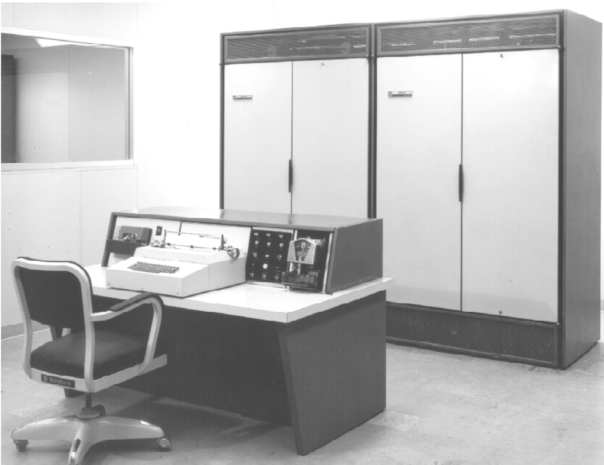
Above - The ADDAPS Programmer's Desk after installation. Notice that P-580 "Elephant Foot" design has been changed to an all-steel design.
