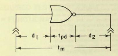
$$t_m = d_1 + t_{pd} + d_2 = t_{pd} + (d_1 + d_2)$$
