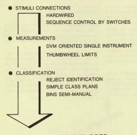
BASIC TECHNIQUES DEVELOPED (AND STILL USED) FOR TRANSISTOR TESTING It wasn't too long before the introduction of more complex devices (initially small scale integration IC's) increased the amount of control and data requirements necessary to manage the test functions.
