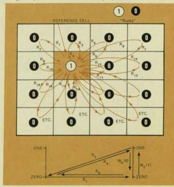
Galloping ONE's pattern tests all possible read/read transitions. It also examines the disturbance caused in other cells by writing in a given cell and provides a rough check of access times between any two cell locations.
