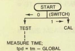
(PERFORM INTERNAL MEASUREMENT AS DEFINED i.e. SET tpd = 0. SAVE RESULT AS GLOBAL VARIABLE) PERFORMED ONCE!
