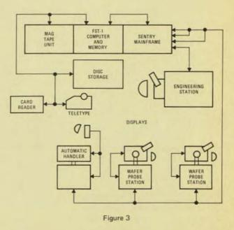
A disc file facilitates program assembly and storage. The file also refreshes the computer memory when long programs are run. About 350 test programs averaging 1,500 instructions each can be stored on disc along with the computer operating systems software.
