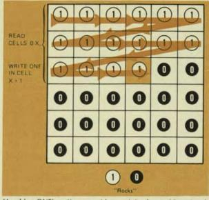
Marching ONE's pattern provides a minimal test of functionality and addressing problems, but is poor at pinpointing difficulties in access times, write recoveries and multiple cell selections. After any test, such as the marching ONE's pattern, is performed, it's often followed by its complement—in this case, a marching ZERO's pattern.
