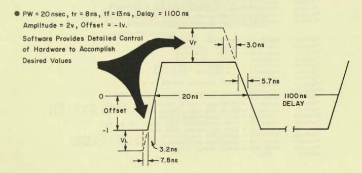
SOFTWARE MANAGES HARDWARE CONTROL REQUIREMENTS & AUTOMATICALLY COMPUTES OFFSETS 19
