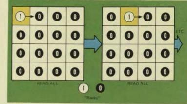
Walking ONE's pattern moves a single bit through the entire grid, providing a good test of the memory's cell addressing. It also detects slow sense-amplifier recovery.
