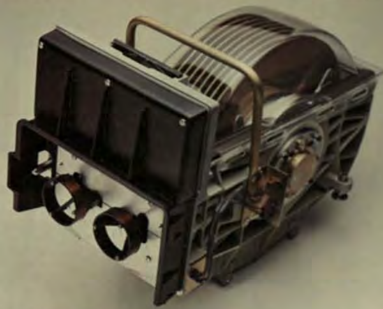
Fig 1 High storage densities are obtained with files employing a head/disk assembly in which the heads and disks are an integral unit. This packaging configuration allows lower head flying heights and thinner media coatings.
