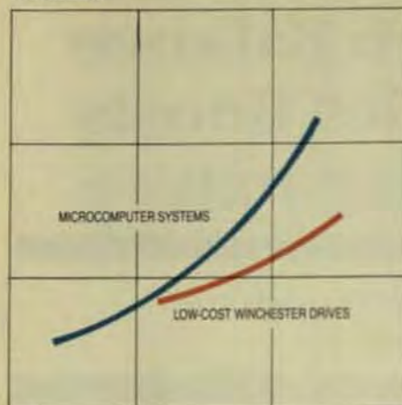
Fig 1 Technology-driven improvements in small computer systems have outpaced developments in mass-storage devices.
