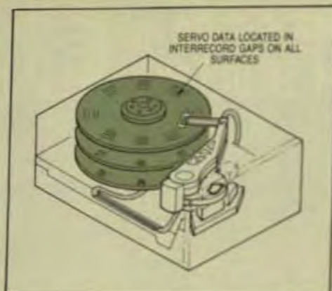
Fig 6 In an embedded-servo system, positioning data is recorded and retrieved in inter-record gaps on every disk surface.
