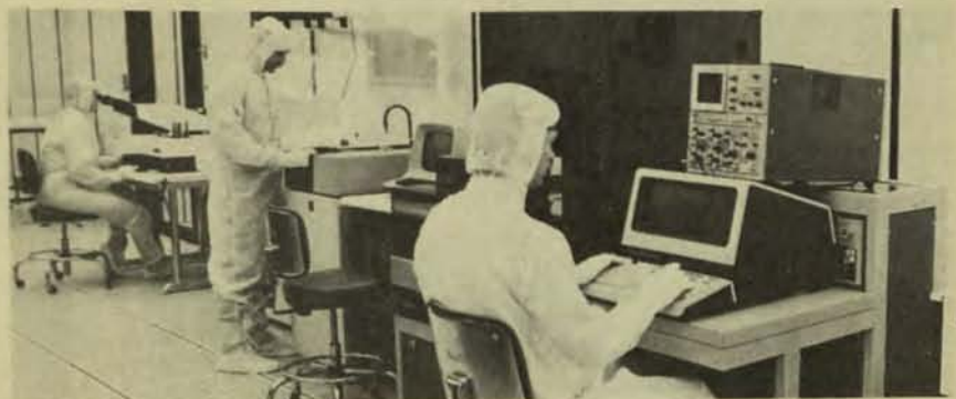
In Gigabit's GaAs factory, says Bryant M. Welch, vice president-manufacturing, "a key feature is our Class 10 clean room." That means dust-particle counts are restricted to fewer than ten particles per cubic foot—and air purity is essential in getting high yields of chips.
