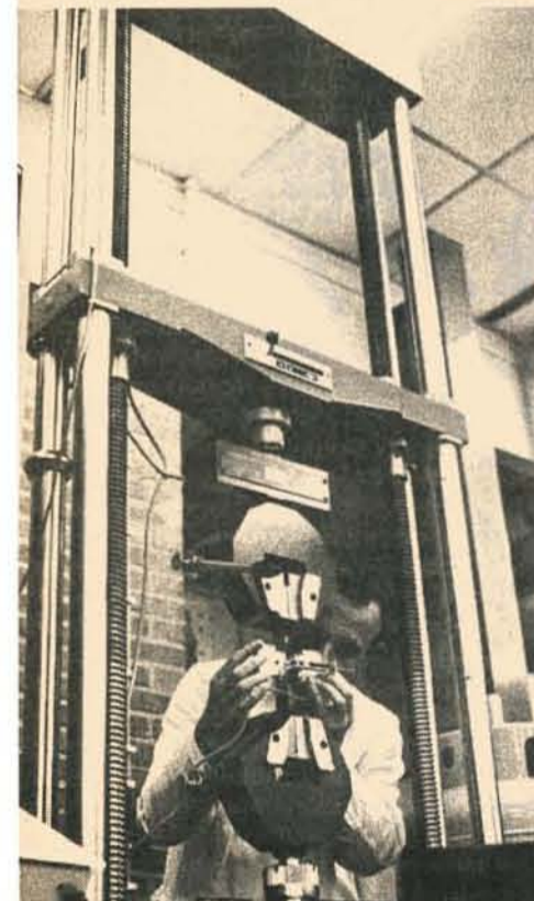
In one of Emmen's well-equipped engineering labs, Bram Casteleyn conducts a tensile strength test.
