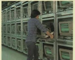
At Tandem's new paperless plant in Austin, each person builds and tests a complete terminal, and "signs" the finished product.
