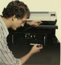
Efficiency of Tandem technical support personnel is enhanced by on-line tools such as the self-contained, microcomputer-based diagnostics console of the NonStop II (above) that is used for on-site and remote trouble-shooting. Customer engineers around the world also use Tandem's corporate EXPAND network to retrieve technical assistance automatically from company headquarters. Low turnover within the Tandem field support organization helps the company
