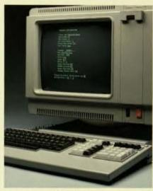
This year Tandem began to manufacture an ergonomic terminal of its own design. The new terminal features user comfort, high throughput, and data integrity. In addition to the 6530 terminal, Tandem introduced a completely new line of higher performance peripheral devices.
