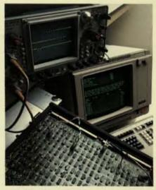
ORACLE, a Tandem-developed system for automatic testing of printed circuit boards introduced into Tandem manufacturing locations during 1982, provides testing functions not previously possible, and dramatically boosts manufacturing productivity. Other manufacturing enhancements brought on-stream during 1982 include new capabilities for automated assembly of printed circuit boards.
