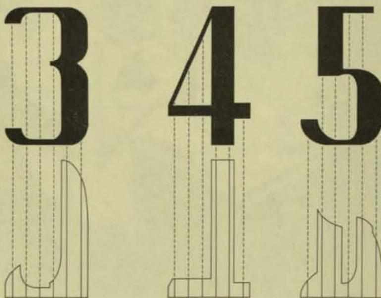
Arabic numerals and the wave forms produced by the Travelers Check scanner. As the numbers printed on the Travelers Check pass horizontally beneath the read-head, the head sums up the total magnetic ink covered in a given time interval and produces a proportional electric signal.
