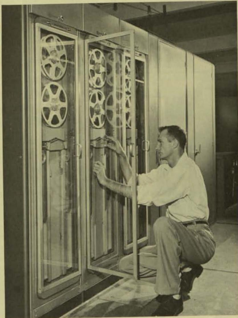
Detailed account activity information is "filed" by ERMA on 10 reels of magnetic tape, each almost half a mile in length. Accounts are kept in numerical order on the tapes which provide storage space for a month's activity.
