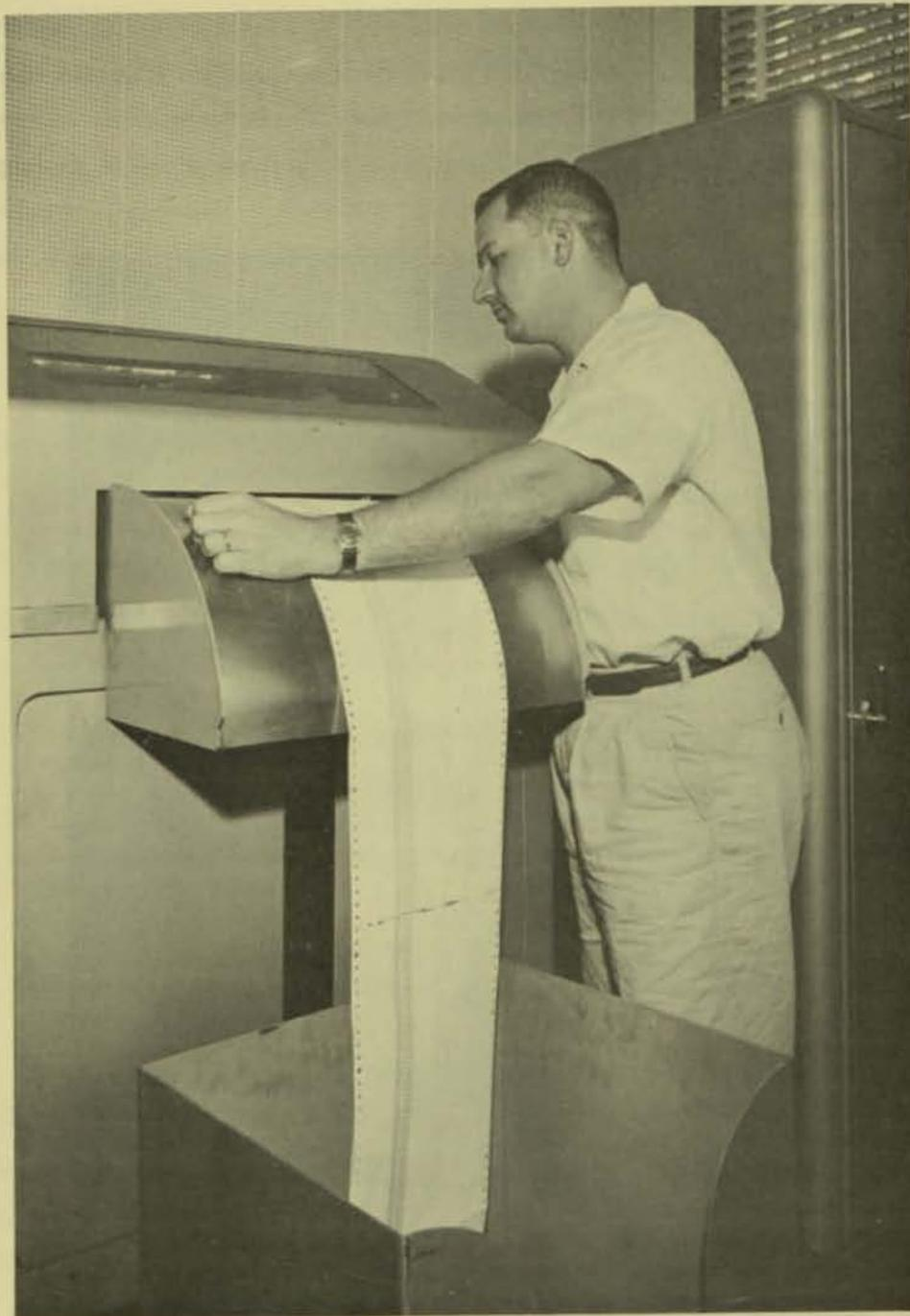
The high speed printer, used in statement preparation, prints 15 lines per second. The printer can prepare all the statements for ten branch banks in about five working days.
