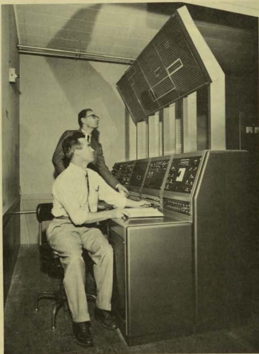
ERMA's "Service Station" used to insure the perfect operation of the many delicate circuits in the bookkeeping machine. This maintenance board facilitates the location of troubles within the machine.
