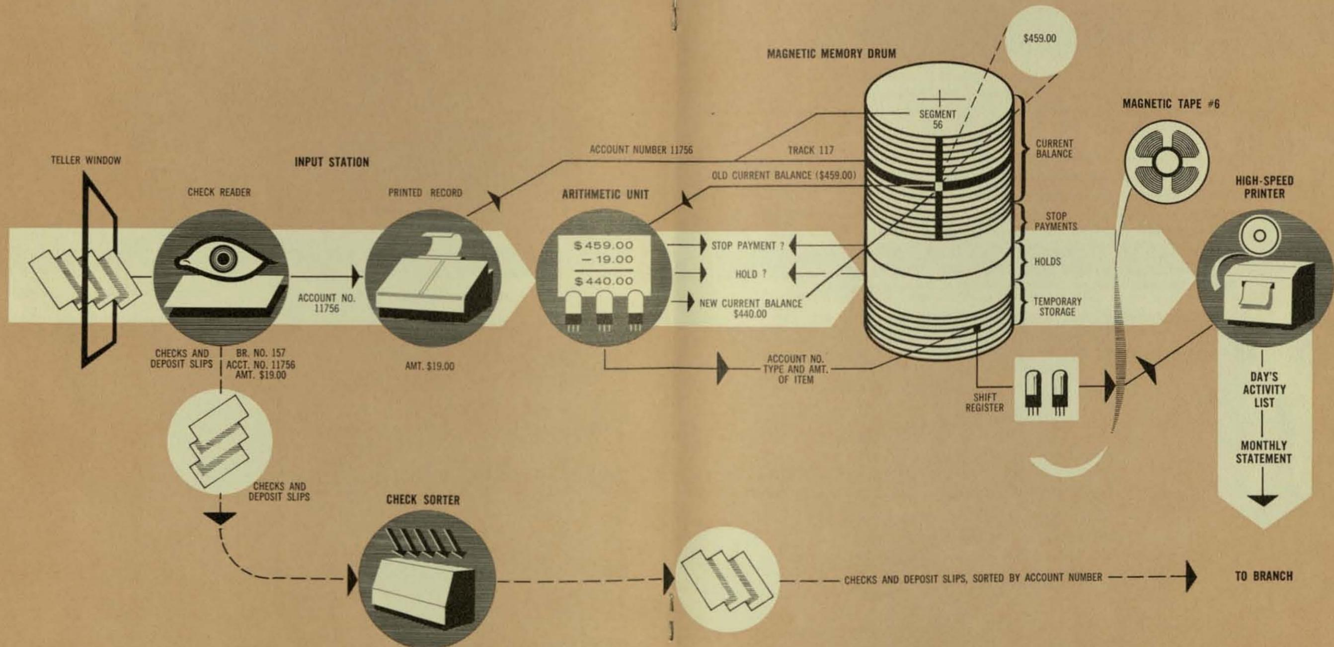
This chart illustrates the processing of checks and deposits by ERMA. The physical check or deposit takes the path of the dotted line; the information from it follows the solid lines. Checks and deposits are received in the normal manner by the ERMA operators. Assume, as a typical case, a check for \$19.00 issued by A. Brown, whose account number is 157 11756. The first three numbers (157) identify the branch where Mr. Brown has his account. To perform the bookkeeping for this check
