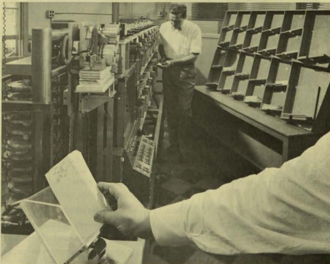
The electronic check sorter separates the checks by account number and by bank branch so the checks may be returned to the customer with his monthly statement. Automatic sorting is made possible by a special magnetic ink code marking on the back of each check.
