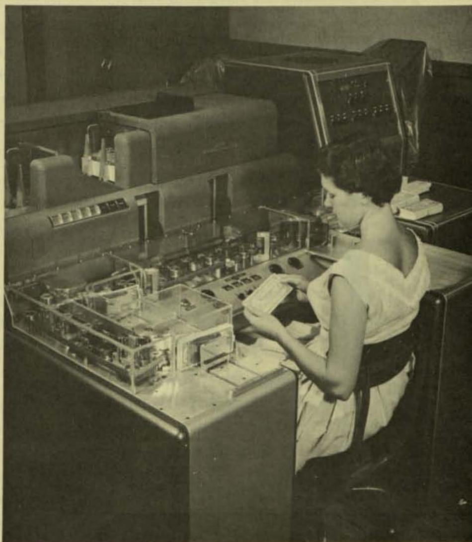
Operator using the Travelers Check number-scanning machine. This machine "reads" arabic numbers on Travelers Checks and punches IBM cards for use in Bank of America accounting systems.
