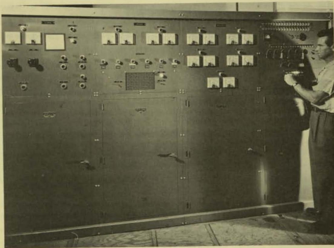
Power at seven different voltages is required to keep ERMA in operation. This panel controls the units required to convert 80 kilowatts of alternating current to direct current and to assure freedom from voltage variations.
