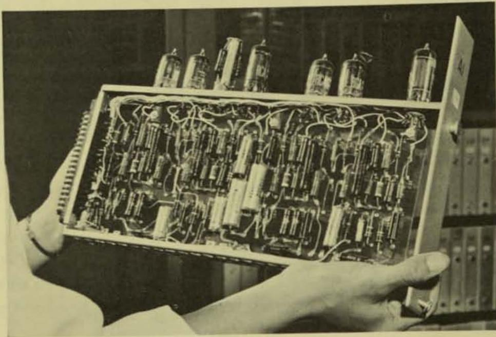
One of the "building blocks" used in the arithmetic unit, capable of performing additions and subtractions on sums as large as \$99,999,999.99.
