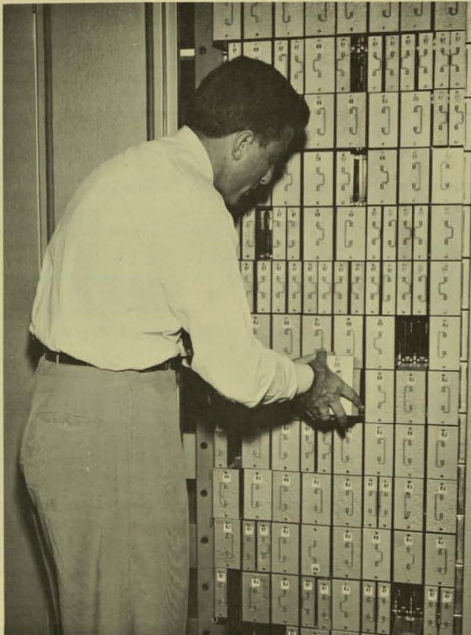
Hundreds of relay units are combined in the construction of ERMA. The units are all of the "plug-in" type and can be replaced with a minimum of difficulty and lost time.
