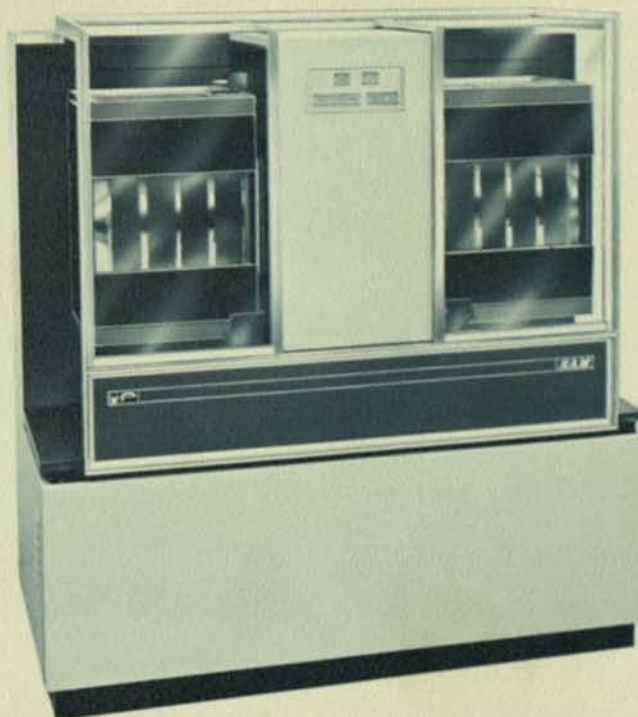
Figure 1. The Potter RAM, Model TLM-4550. Shown with Model ACC-8601 Tape Pack Cartridge
