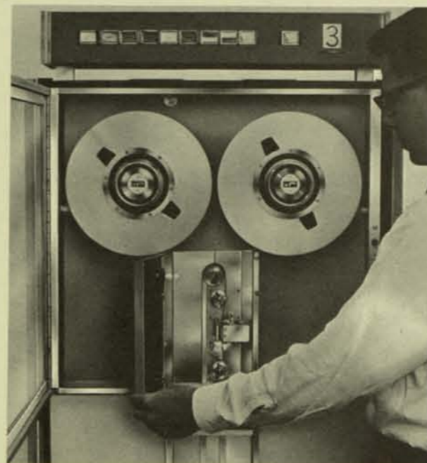
Figure 5. Simplified Tape Loading
