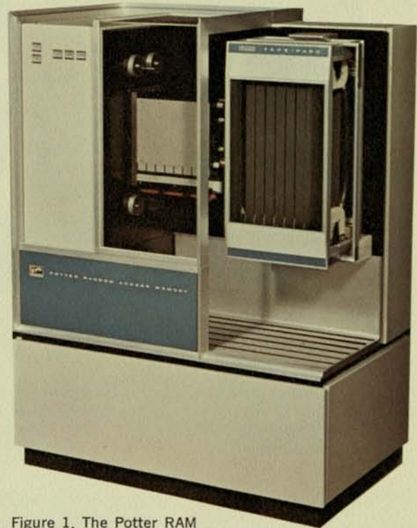
Figure 1. The Potter RAM (a random access memory system) Model TLM-4505, Shown with Model ACC-8606 Cartridge
