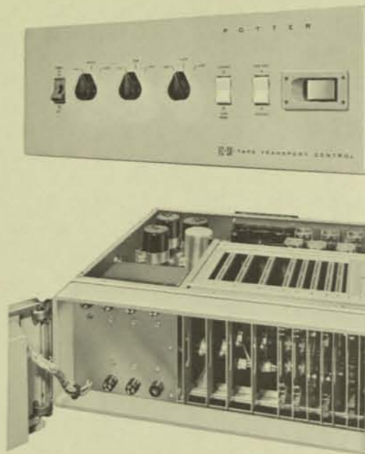
Figure 3. Potter EC-SR Drive Electronics and Control Assembly
