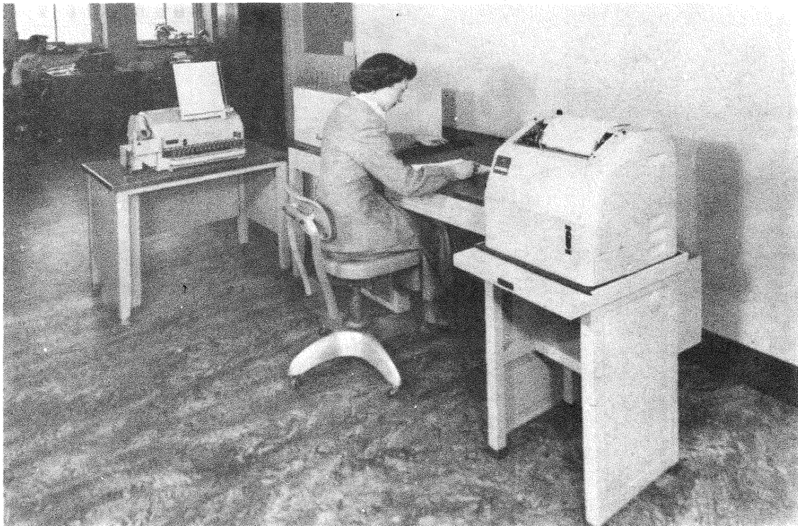
Fig. 8. An operator station for the Model VI relay computer. (Andrews, Electrical Engineering , September 1949, p.752)
