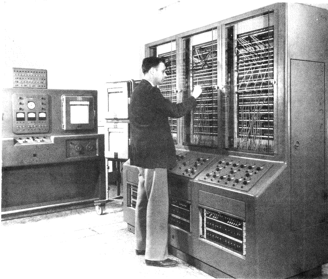
Fig. 1. Richard W. Hamming setting up a problem on the general purpose analog computer — nicknamed Gypsy.
