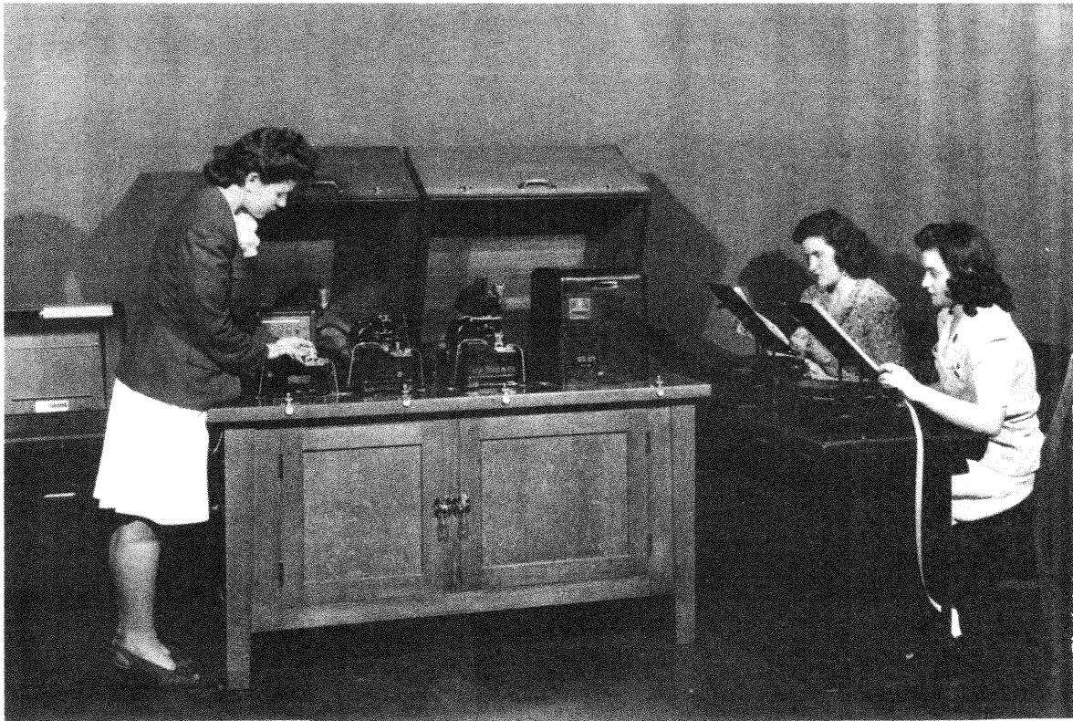
Fig. 6. Paper-tape terminal for the ballistic computer. (Randell, Origins of Digital Computers , p.251)
