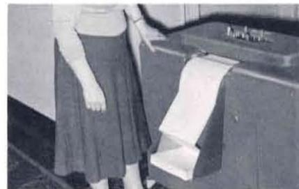
D. Listomatic Camera photographs cards onto continuous film.
